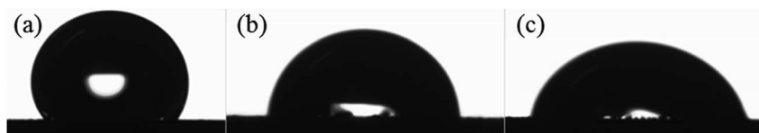
Fig. 3 Contact angle formed by water droplets on (a) AC: \theta = 124.63^\circ \pm 3.1 , (b) AC-HDTMA: \theta = 87.47^\circ \pm 2.7 , (c) AC-T80-HDTMA: \theta = 76.61^\circ \pm 2.9 .
