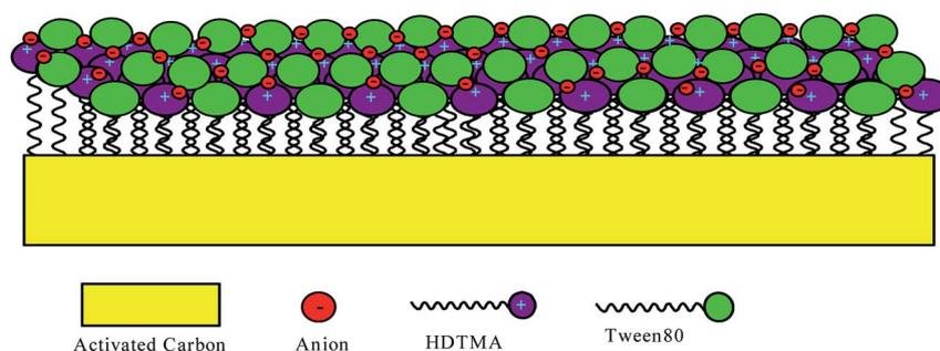
Fig. 9 Adsorption of anions on functionalized AC electrode.
