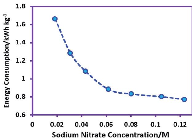
Fig. 4 Variation of energy consumption with the sodium nitrate concentration.
