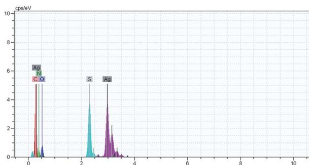
Fig. 8 EDS spectrum of as synthesized silver sulfadiazine.
