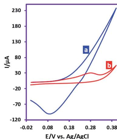
Fig. 1 Cyclic voltammograms of silver electrode (area, 1.8 mm<sup>2</sup>), (a) in the absence and (b) in the presence of sulfadiazine (10 mM). Scan rate: 100 mV s<sup>-1</sup>. Temperature: 25 ± 1 °C.
