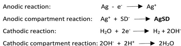
Scheme 1 Reaction mechanism for electrochemical synthesis of AgSD.
