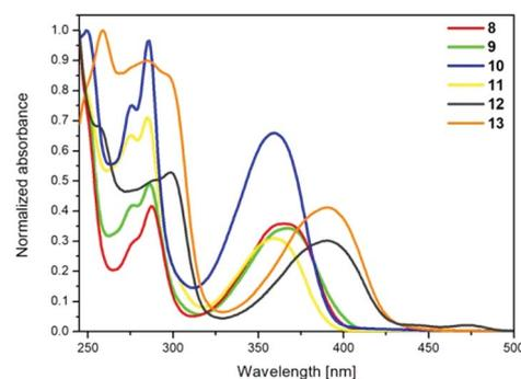
Fig. 3 Absorption spectra recorded for **8–13** in a CH<sub>2</sub>Cl<sub>2</sub> solution ( $c = 10^{-5} \text{ mol L}^{-1}$ ).
