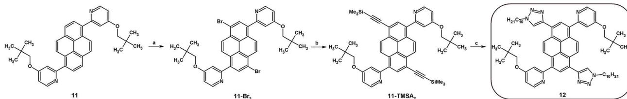
**Scheme 2** Synthesis of tetrasubstituted pyrene derivative **12**. *Reagents and conditions:* (a)  $\text{Br}_2$ ,  $\text{CH}_2\text{Cl}_2$ ,  $40^\circ\text{C}$ , 2 h; (b) TMSA,  $[\text{Pd}(\text{PPh}_3)_4]$ ,  $\text{CuI}$ ,  $\text{NEt}_3$ , DBU,  $90^\circ\text{C}$ , 16 h; (c) decyl azide,  $\text{KF}$ ,  $\text{CuSO}_4 \cdot 5\text{H}_2\text{O}$ , sodium ascorbate, pyridine,  $\text{EtOH}$ ,  $\text{H}_2\text{O}$ , room temp., 24 h.
