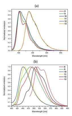
Fig. 4 Emission spectra recorded from (a) a  $CH_2Cl_2$  solution (c =  $10^{-5}$  mol L<sup>-1</sup>) and (b) the solid state for 8-13.
