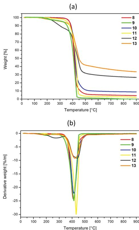
**Fig. 2** TGA (a) and DTG (b) curves for **8–13**.
