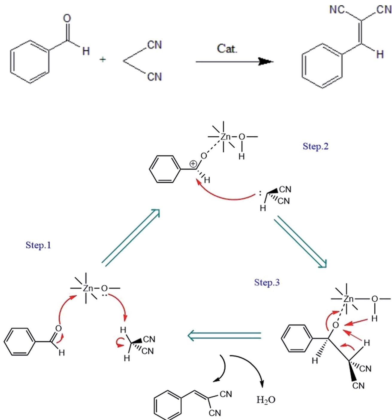
Fig. 5 The scheme catalytic mechanism of Knoevenagel condensation reaction.
