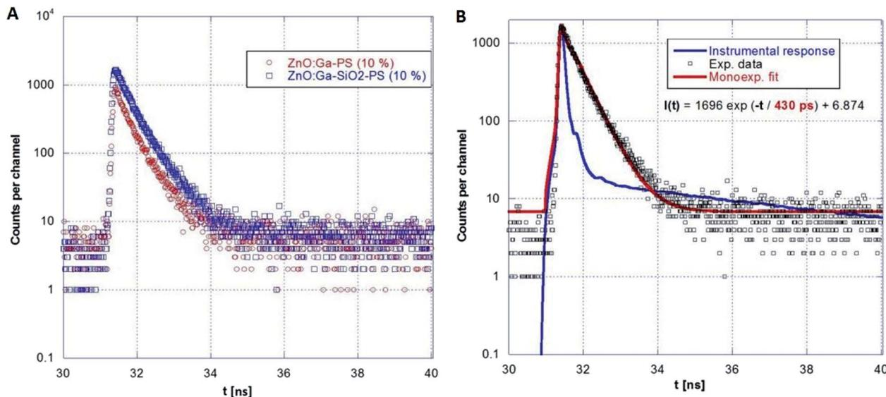
Fig. 10 Comparison of ZnO:Ga-PS (10 wt%) and ZnO:Ga-SiO<sub>2</sub>-PS (10 wt%) RL decays (A) and single-exponential fit for ZnO:Ga-SiO<sub>2</sub>-PS (10 wt%) sample (B).
