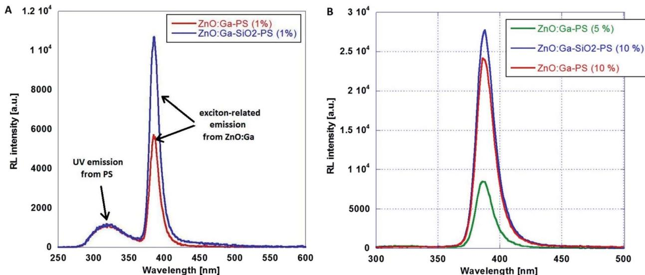
Fig. 8 RL spectra of ZnO:Ga-PS (1 wt%) and ZnO:Ga-SiO<sub>2</sub>-PS (1 wt%) composites (A) and composites with 5 wt% and 10 wt% filling (B).
