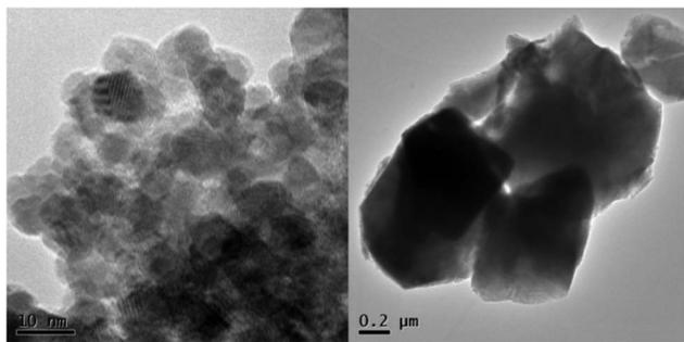
Fig. 2 HRTEM images of ZnO:Ga-SiO<sub>2</sub> without further heat treatment (left) and after treatment at 1000 °C (right).
