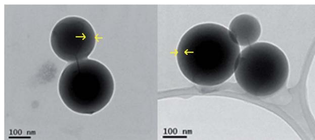
Fig. 5 HRTEM images of ZnO:Ga-SiO<sub>2</sub> core-shells. Arrows denote thickness of SiO<sub>2</sub> shell.
