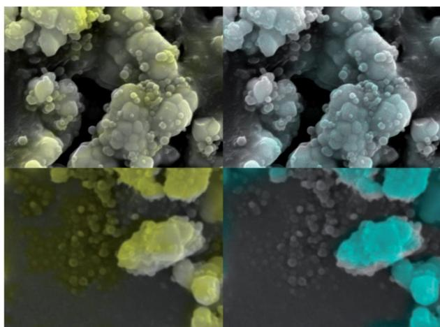
Fig. 4 SEM images of ZnO:Ga-SiO<sub>2</sub> particles with EDX element analysis. Turquoise colour represents zinc, yellow colour represents silicon.
