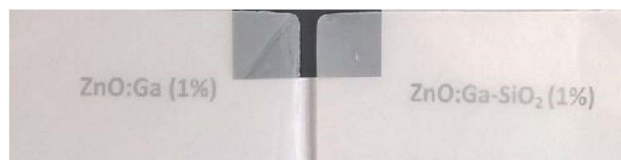
Fig. 7 Images of 1 mm thick ZnO:Ga-PS composite plates (1 wt% filling).
