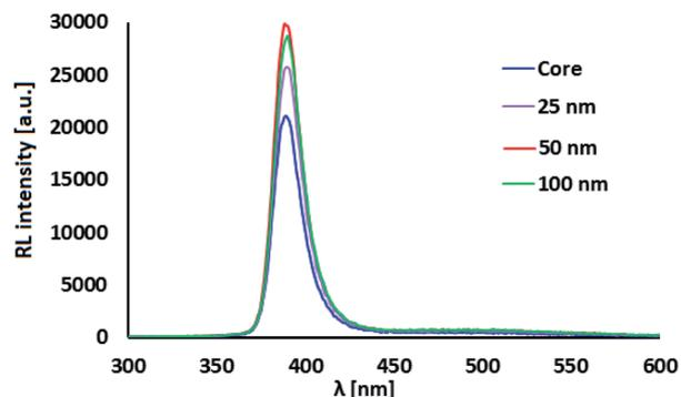
Fig. 6 RL spectra of ZnO:Ga-SiO<sub>2</sub> with different SiO<sub>2</sub> theoretical thickness.
