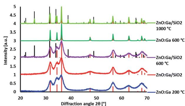
Fig. 1 XRPD diffractograms of ZnO:Ga and ZnO:Ga-SiO<sub>2</sub> heat treated at various temperatures. Diffraction lines of ZnO PDF database record #00-036-1451 given by red dashed lines, Zn<sub>2</sub>SiO<sub>4</sub> PDF database record #00-037-1485 given by black dashed lines.
