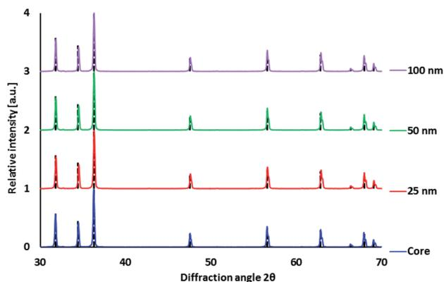
Fig. 3 XRPD diffractograms of ZnO:Ga-SiO<sub>2</sub> (ZnO:Ga annealed at 1000 °C before coating) with different SiO<sub>2</sub> theoretical thickness. Diffraction lines of ZnO PDF database record #00-036-1451 given by black dashed lines.
