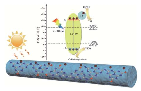
Schematic diagram for charge separation and transfer and H<sub>2</sub> evolution mechanism of the OCN under visible-light irradiation.
