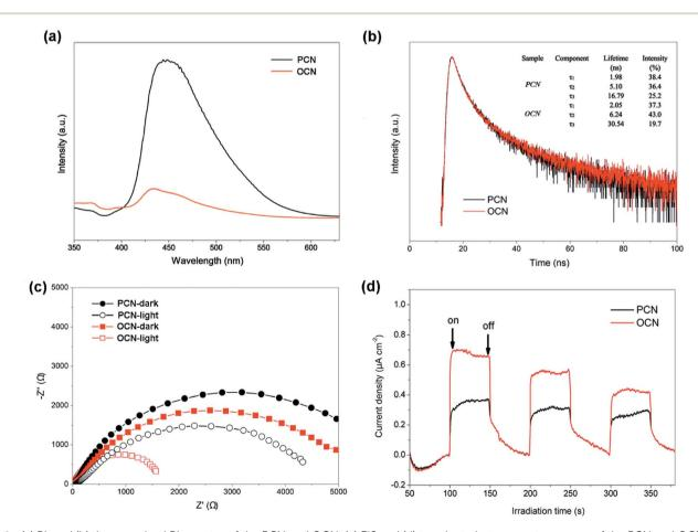
Fig. 8 (a) PL and (b) time-resolved PL spectra of the PCN and OCN. (c) EIS and (d) transient photocurrent response of the PCN and OCN with/ without visible-light irradiation ( $\lambda > 400$  nm).
