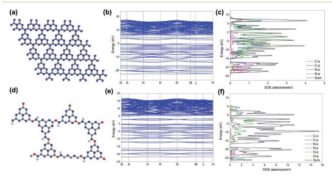
Fig. 6 (a and d) Structure models of the PCN and OCN (gray: C; blue: N; red: O). (b and e) Calculated band structures and (c and f) corresponding PDOS for the PCN and OCN, respectively.
