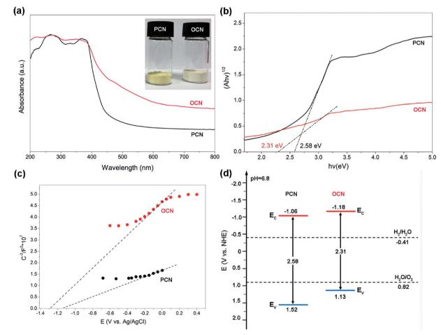
Fig. 5 (a) UV-vis DRS spectra and (b) Tauc plots of  $(\alpha h v)^{1/2}$  vs. photon energy for band gap calculations of the PCN and OCN. Inset shows a digital photograph of the PCN (left) and OCN (right). (c) Mott–Schottky plots and (d) band structure diagram for the PCN and OCN.
