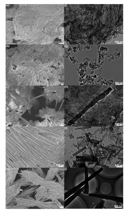
Fig. 4 (a-e) FESEM and (f-j) TEM images of the samples obtained at different hydrothermal times: (a and f) 3 h, (b and g) 6 h, (c and h) 9 h, (d and i) 12 h and (e and j) 24 h.
