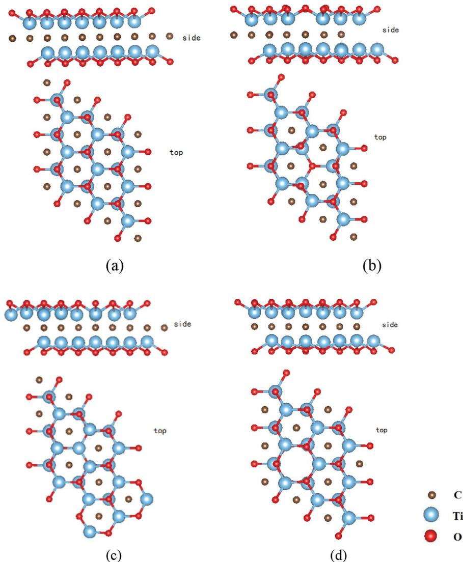
Fig. 1 The atomic structures of pristine  $\text{Ti}_2\text{CO}_2$  (a),  $\text{Ti}_2\text{CO}_2\text{-V}_{\text{Ti}}$  (b),  $\text{Ti}_2\text{CO}_2\text{-V}_{\text{O}}$  (c), and  $\text{Ti}_2\text{CO}_2\text{-V}_{\text{C}}$  (d) from top and side view.
