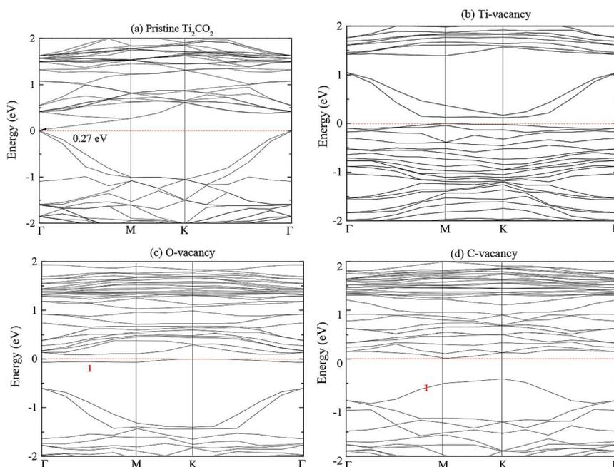
Fig. 2 The band structure of pristine and vacancy defect Ti<sub>2</sub>CO<sub>2</sub> monolayer.
