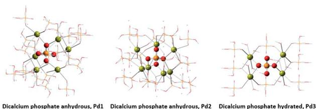
Fig. 8 Crystallographic structures by molecular modelling of DCP.
