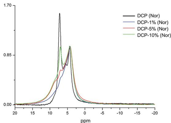
Fig. 7 Superimposition of  $^{31}\text{P}$  NMR spectra of DCP fertilizer samples prepared at different amounts of aqueous potassium humate (1, 5 and 10%). The intensities are normalized with respect to the signal at 4.20 ppm.
