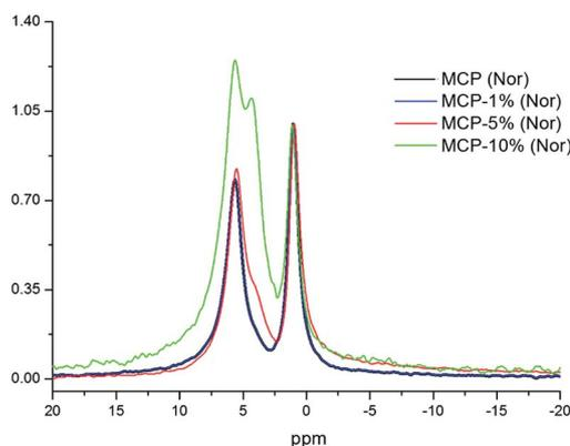
Fig. 2 Superimposition of 1D <sup>31</sup>P NMR spectra of MCP fertilizer samples prepared at different amounts of aqueous potassium humate (1, 5 and 10%). The intensities are normalized with respect to the signal at 1.12 ppm.
