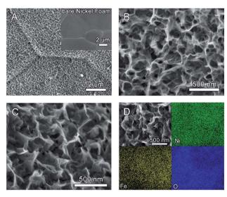
Fig. 1 (A and B) SEM images of different magnifications for  $Ni(OH)_2$  nanosheets grown from nickel foam (inset is SEM image of a bare nickel foam). (C) SEM and (D) SEM-EDX mapping images of the  $Ni(OH)_2$ -Fe/NF electrode.
