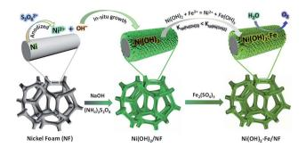
Scheme 1 Fabrication process of the Ni(OH)<sub>2</sub>–Fe electrodes and their utilization for water oxidation
