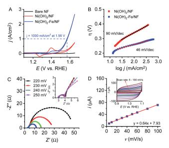
Fig. 3 (A) CV plots of a bare nickel foam (NF), Ni(OH)<sub>2</sub>/NF and Ni(OH)<sub>2</sub>-Fe/NF electrodes. (B) Tafel plots of the Ni(OH)<sub>2</sub>-Fe/NF and Ni(OH)<sub>2</sub>-Fe/NF electrodes. (C) Nyquist plots of Ni(OH)<sub>2</sub>-Fe/NF electrode at various overpotentials; inset shows the high-frequency regions. (D) The anodic charging current at 1.0 V vs. RHE, plotted against the scan rates of Ni(OH)<sub>2</sub>-Fe/NF electrode; inset shows the corresponding CVs curves.
