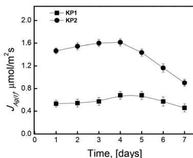
Fig. 12 The flux transport of Ag(I) ions calculated obtained for long-term transport across SLM. Source phase:  $5.0 \times 10^{-4}$  M  $\text{AgNO}_3$ , pH = 4.0; membrane:  $4.0 \text{ cm}^3$  *o*-NPPE/1.0 g CTA; 0.10 M KP1 and KP2, receiving phase: 0.10 M  $\text{Na}_2\text{S}_2\text{O}_3$ .
