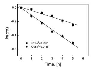
Fig. 3 The relationship  $ln(c/c_i)$  vs. time transport of ions Ag(i) across PIM with KP1 and KP2. Source phase:  $5.0 \times 10^{-4}$  M AgNO<sub>3</sub>, pH = 4.0; membrane: 2.0 cm<sup>3</sup> o-NPPE/1.0 g CTA; 0.10 M KP1 and KP2, receiving phase: 0.10 M Na<sub>2</sub>S<sub>2</sub>O<sub>3</sub>. PIMs compositions were 67% plasticizer, 30% support, 3% KP1; and 63% plasticizer, 31% support, 6% KP2.
