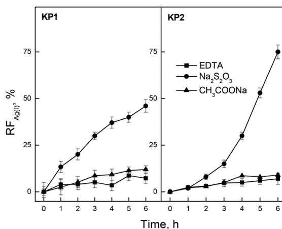
Fig. 6 The recovery factor (RF) obtained for the transport of ions Ag(i) across PIM. Source phase:  $5.0 \times 10^{-4}$  M AgNO<sub>3</sub>, pH = 4.0; membrane: 2.0 cm<sup>3</sup> o-NPPE/1.0 g CTA; 0.10 M KP1 and KP2, receiving phase: 0.10 M EDTA; 0.10 M Na<sub>2</sub>S<sub>2</sub>O<sub>3</sub> and 0.10 M CH<sub>3</sub>COONa. PIMs compositions were 67% plasticizer, 30% support, 3% KP1; and 63% plasticizer, 31% support, 6% KP2.
