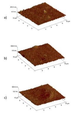
Fig. 13 3D-atomic force microscopy (AFM) images of PIM without carrier (a), PIM containing KP1 (b) as well as PIM containing KP2 (c).
