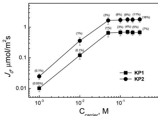
Fig. 7 The Ag(I) transport fluxes vs. ion carrier concentration PIM. Source phase: 1.0 × 10<sup>-3</sup> M AgNO<sub>3</sub>, pH = 4.0; membrane: 2.0 cm<sup>3</sup> *o*-NPPE/1.0 g CTA (carrier concentration expressed in percentage by mass); receiving phase: 0.10 M Na<sub>2</sub>S<sub>2</sub>O<sub>3</sub>.
