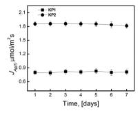
Fig. 11 Changes of the Ag(i) flux during transport across PIM - 7 cycles of measurement. Source phase:  $5.0 \times 10^{-4}$  M AgNO<sub>3</sub>, pH = 4.0; membrane:  $4.0 \text{ cm}^3$  o-NPPE/1.0 g CTA; 0.10 M KP1 and KP2, receiving phase:  $0.10 \text{ M Na}_2\text{S}_2\text{O}_3$ .
