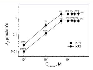
Fig. 7 The Ag(I) transport fluxes vs. ion carrier concentration PIM. Source phase:  $1.0 \times 10^{-3}$  M AgNO<sub>3</sub>, pH = 4.0; membrane: 2.0 cm<sup>3</sup> o-NPPE/1.0 g CTA (carrier concentration expressed in percentage by mass); receiving phase: 0.10 M Na<sub>2</sub>S<sub>2</sub>O<sub>3</sub>.
