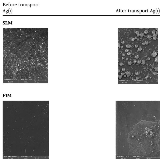
On all membranes containing KP1 and KP2, well-formed inclusions in the polymer of the matrix containing carrier in the plasticizer solution can be seen. In the case of the polymer
