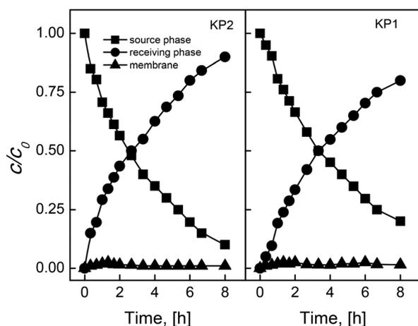
Fig. 2 The profile of Ag(I) concentrations in source, membrane and receiving phases during the transport process across PIMs containing KP1 and KP2. Source phase:  $5.0 \times 10^{-4}$  M AgNO<sub>3</sub>, pH = 4.0; membrane:  $2.0 \text{ cm}^3$  o-NPPE/1.0 g CTA; 0.10 M carrier, receiving phase: 0.10 M Na<sub>2</sub>S<sub>2</sub>O<sub>3</sub>. PIMs compositions were 67% plasticizer, 30% support, 3% KP1; and 63% plasticizer, 31% support, 6% KP2.
