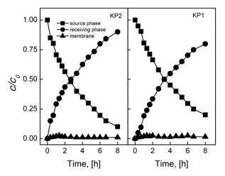
Fig. 2 The profile of Ag(ı) concentrations in source, membrane and receiving phases during the transport process across PIMs containing KP1 and KP2. Source phase:  $5.0 \times 10^{-4}$  M AgNO<sub>3</sub>, pH = 4.0; membrane: 2.0 cm<sup>3</sup> o-NPPE/1.0 g CTA; 0.10 M carrier, receiving phase: 0.10 M Na<sub>2</sub>S<sub>2</sub>O<sub>3</sub>. PIMs compositions were 67% plasticizer, 30% support, 3% KP1; and 63% plasticizer, 31% support, 6% KP2.
