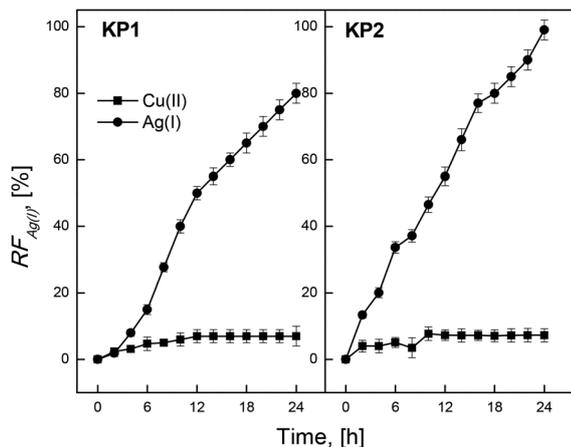
Fig. 10 The relationship of recovery factor (RF) of Ag(i) and Cu(ii) vs. time of the transport through PIM. Source phase:  $5.0 \times 10^{-4}$  M AgNO<sub>3</sub> and Cu(NO<sub>3</sub>)<sub>2</sub>, pH = 4.0; membrane: 4.0 cm<sup>3</sup> *o*-NPPE/1.0 g CTA; 0.10 M KP1 and KP2, receiving phase: 0.10 M Na<sub>2</sub>S<sub>2</sub>O<sub>3</sub>.
