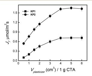
Fig. 9 The effect of o-NPPE plasticizer on the Ag(i) transport through PIM. Source phase:  $5.0\times10^{-4}$  M AgNO<sub>3</sub>, pH = 4.0; membrane: 25.0 mg CTA; 0.10 M KP1 and KP2, receiving phase: 0.10 M Na<sub>2</sub>S<sub>2</sub>O<sub>3</sub>.
