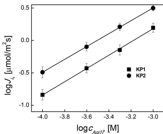
Fig. 5 Logarithmic relation of initial fluxes vs. Ag(i) concentration in the source aqueous phase. Source phase: various concentration of AgNO<sub>3</sub>, pH = 4.0; membrane: 2.0 cm<sup>3</sup> o-NPPE/1.0 g CTA; 0.10 M KP1 and KP2, receiving phase: 0.10 M Na<sub>2</sub>S<sub>2</sub>O<sub>3</sub>. PIMs compositions were 67% plasticizer, 30% support, 3% KP1; and 63% plasticizer, 31% support, 6% KP2.
