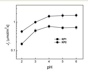
Fig. 4 The relationship of the initial ion flux transport Aq(I) across the PIM vs. the pH of the source phase. Source phase:  $5.0 \times 10^{-4}$  M AgNO<sub>3</sub>; membrane:  $2.0 \text{ cm}^3 \text{ o-NPPE/1.0 g CTA}$ ; 0.10 M KP1 and KP2, receiving phase: 0.10 M Na<sub>2</sub>S<sub>2</sub>O<sub>3</sub>. PIMs compositions were 67% plasticizer, 30% support, 3% KP1; and 63% plasticizer, 31% support, 6% KP2.
