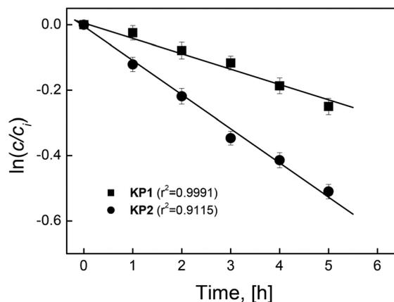
Fig. 3 The relationship  $\ln(c/c_i)$  vs. time transport of ions Ag(I) across PIM with KP1 and KP2. Source phase:  $5.0 \times 10^{-4}$  M AgNO<sub>3</sub>, pH = 4.0; membrane:  $2.0 \text{ cm}^3$  o-NPPE/1.0 g CTA; 0.10 M KP1 and KP2, receiving phase: 0.10 M Na<sub>2</sub>S<sub>2</sub>O<sub>3</sub>. PIMs compositions were 67% plasticizer, 30% support, 3% KP1; and 63% plasticizer, 31% support, 6% KP2.
