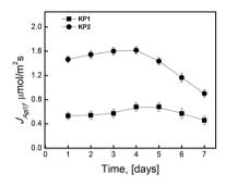
Fig. 12 The flux transport of Ag(I) ions calculated obtained for long-term transport across SLM. Source phase:  $5.0 \times 10^{-4}$  M AgNO<sub>3</sub>, pH = 4.0; membrane: 4.0 cm<sup>3</sup> o-NPPE/1.0 g CTA; 0.10 M KP1 and KP2, receiving phase: 0.10 M Na<sub>2</sub>S<sub>2</sub>O<sub>3</sub>.
