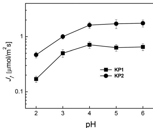
Fig. 4 The relationship of the initial ion flux transport Ag(I) across the PIM vs. the pH of the source phase. Source phase:  $5.0 \times 10^{-4}$  M AgNO<sub>3</sub>; membrane:  $2.0 \text{ cm}^3$  o-NPPE/1.0 g CTA; 0.10 M KP1 and KP2, receiving phase: 0.10 M Na<sub>2</sub>S<sub>2</sub>O<sub>3</sub>. PIMs compositions were 67% plasticizer, 30% support, 3% KP1; and 63% plasticizer, 31% support, 6% KP2.
