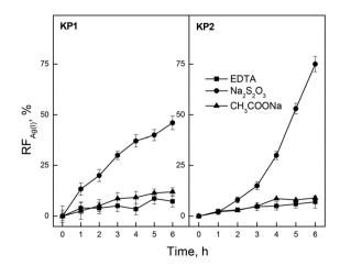
Fig. 6 The recovery factor (RF) obtained for the transport of ions Ag(I) across PIM. Source phase:  $5.0 \times 10^{-4}$  M AgNO<sub>3</sub>, pH = 4.0; membrane:  $2.0 \text{ cm}^3$  o-NPPE/1.0 g CTA; 0.10 M KP1 and KP2, receiving phase: 0.10 M EDTA; 0.10 M Na<sub>2</sub>S<sub>2</sub>O<sub>3</sub> and 0.10 M CH<sub>3</sub>COONa. PIMs compositions were 67% plasticizer, 30% support, 3% KP1; and 63% plasticizer, 31% support, 6% KP2.
