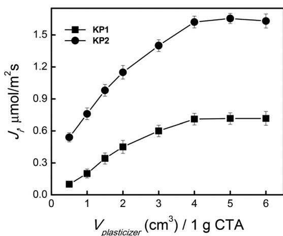
Fig. 9 The effect of *o*-NPPE plasticizer on the  $\text{Ag}(\text{i})$  transport through PIM. Source phase:  $5.0 \times 10^{-4} \text{ M}$   $\text{AgNO}_3$ , pH = 4.0; membrane: 25.0 mg CTA; 0.10 M **KP1** and **KP2**, receiving phase: 0.10 M  $\text{Na}_2\text{S}_2\text{O}_3$ .
