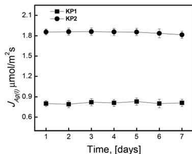
Fig. 11 Changes of the Ag(I) flux during transport across PIM – 7 cycles of measurement. Source phase:  $5.0 \times 10^{-4}$  M  $\text{AgNO}_3$ , pH = 4.0; membrane:  $4.0 \text{ cm}^3$  *o*-NPPE/1.0 g CTA; 0.10 M KP1 and KP2, receiving phase: 0.10 M  $\text{Na}_2\text{S}_2\text{O}_3$ .
