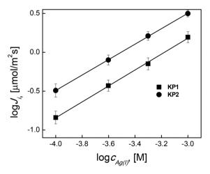
Fig. 5 Logarithmic relation of initial fluxes vs. Ag(i) concentration in the source aqueous phase. Source phase: various concentration of AgNO<sub>3</sub>, pH = 4.0; membrane: 2.0 cm<sup>3</sup>  $\sigma$ -NPPE/1.0 g CTA; 0.10 M KP1 and KP2, receiving phase: 0.10 M Na<sub>2</sub>S<sub>2</sub>O<sub>3</sub>. PlMs compositions were 67% plasticizer, 30% support, 3% KP1; and 63% plasticizer, 31% support, 6% KP2.
