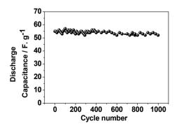
Fig. 12 Cycling stability of the calcined chicken eggshell at 900  $^{\circ}$ C exhibiting a discharge capacitance of 55 F g<sup>-1</sup> having a retention of 100% after 1000 cycles.
