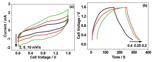
Fig. 14 Symmetrical supercapacitor comprising chicken eggshell as-crushed against calcined at 900 °C. (a) CV curves; and (b) chargedischarge profiles exhibiting a capacitor behaviour. The sweep rates and current density (A  $g^{-1}$ ) are given in the respective figures.
