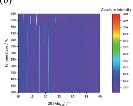
Fig. 2 (a) X-ray diffraction (XRD), and (b) corresponding top view of the patterns of chicken eggshell synthesized from room temperature to 900 °C, various profiles are stacked in the image.
