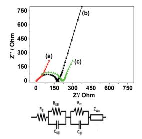
Fig. 11 Nyquist plot comparing the impedance in high frequency region and capacitive/battery behaviour in low frequency region for chicken eggshell (a) as-crushed; and calcined at: (b) 600  $^{\circ}$ C and (c) 900  $^{\circ}$ C. The capacitive and battery type behaviour is seen for 600  $^{\circ}$ C and 900  $^{\circ}$ C, respectively. The corresponding equivalent circuit is shown below the plot.
