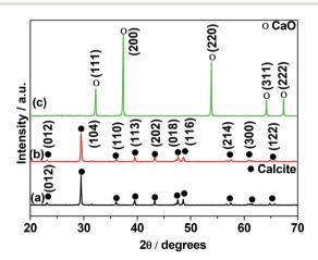
Fig. 1 X-ray diffraction (XRD) patterns of chicken eggshell (a) ascrushed; and calcined at: (b) 600 °C and (c) 900 °C. The lower temperature CaCO<sub>3</sub> material displayed a much weaker pattern, suggesting it was not a much crystalline
