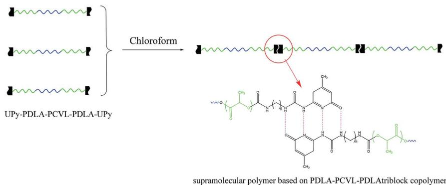
Scheme 1 Synthetic route of supramolecular polymers based on PDLA-PCVL-PDLA triblock copolymers.
