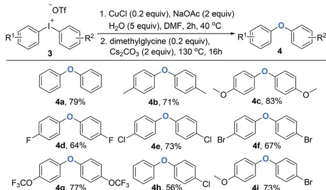
**Scheme 3** One-pot synthesis of diaryl ethers from diaryliodoniums. Reaction conditions: (1) **1** (0.2 mmol), CuCl (10 mol%), NaOAc (2 equiv.), H<sub>2</sub>O (5 equiv.), DMF (1.0 mL), Ar, 40 °C, 2 h; (2) Cs<sub>2</sub>CO<sub>3</sub> (2 equiv.) and dimethylglycine (0.2 equiv.) were added, Ar, 130 °C, 16 h.
