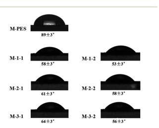
Water contact angles for M-PES and the modified membranes.
