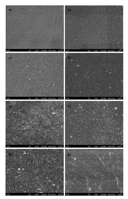
Fig. 3 SEM images of the surface morphologies for (a) and (b) M-PES, (c) M-1-1, (d) M-1-2, (e) M-2-1, (f) M-2-2, (g) M-3-1, and (h) M-3-2.
