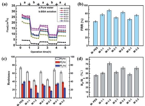
Fig. 6 Anti-fouling properties of the membranes: (a) time-dependent fluxes, (b) water flux recovery ratios (FRR), (c) resistances, and (d) ratio of irreversible fouling ( $R_t$ ) to total fouling ( $R_t$ ).
