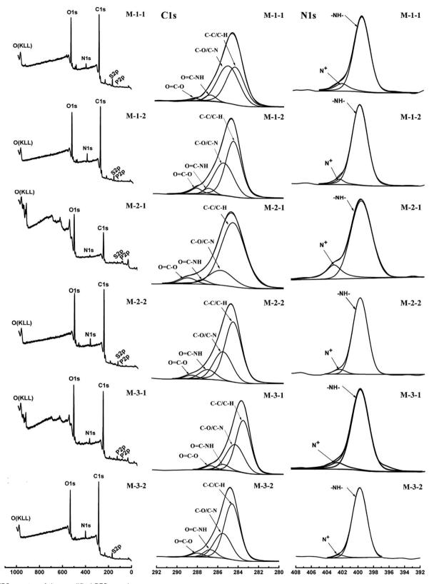
Fig. 2 XPS spectra of the modified PES membranes.
