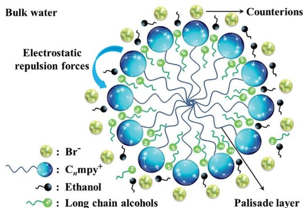
Fig. 5 Schematic illustration of  $[C_nmpy][Br]$  micelle in the presence of inorganic salts and organic alcohols in water.
