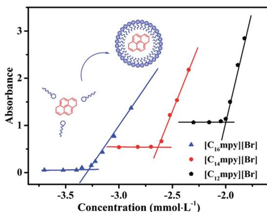
**Fig. 4** The plots of absorption intensity vs. concentration of  $[C_n\text{mpy}][\text{Br}]$  at 338 nm.
