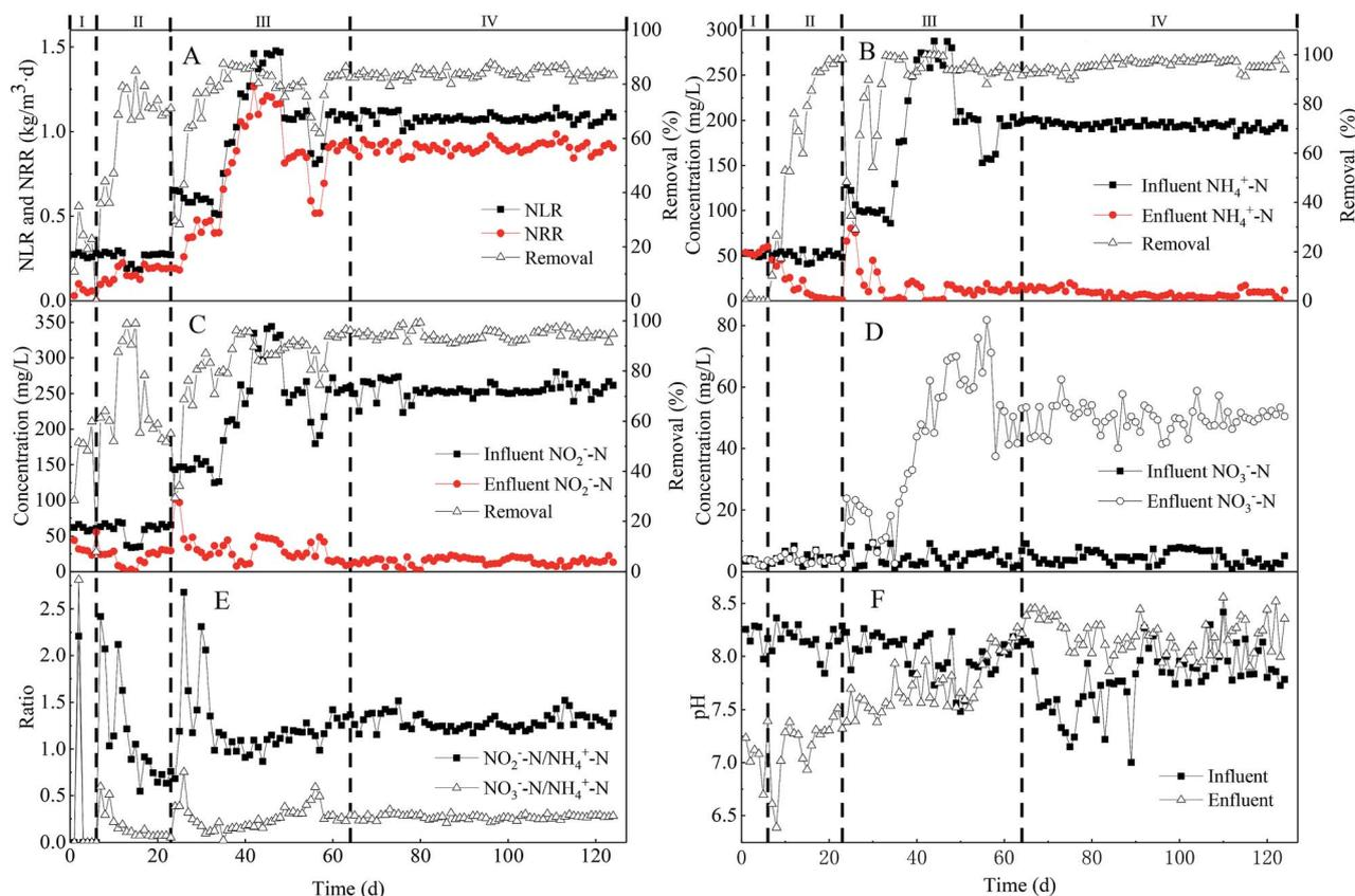
Fig. 2 Start-up and long-term performance of the UPPAR: (A) nitrogen loading and removal rate; (B)  $\text{NH}_4^+\text{-N}$  removal efficiency; (C)  $\text{NO}_2^-\text{-N}$  uptake efficiency; (D) nitrate production and accumulation; (E) stoichiometric ratio; (F) pH profile.
