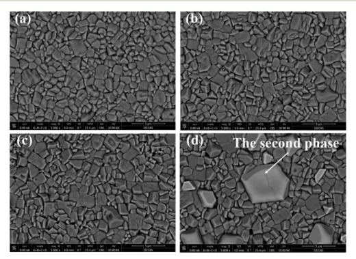
Fig. 2 The scanning electron microscopy photographs of xNb doped BNT-BKT ceramics with (a) x = 1%, (b) x = 3%, (c) x = 5%, (d) x = 7%.
