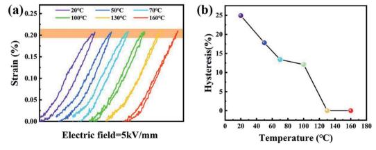
Fig. 6 The temperature dependent (a) the strain value of 5Nb ceramics and (b) the corresponding hysteresis
