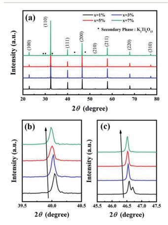
Fig. 1 (a) XRD patterns of xNb ceramics. (b and c) Enlarged (111) and (200) peaks around  $40^{\circ}$  and  $46^{\circ}$ , respectively.
