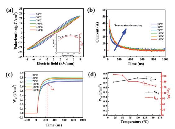
Fig. 9 (a) The temperature dependent P-E loops of 5Nb ceramics at 8 kV mm<sup>-1</sup>, the inset shows corresponding  $W_{\rm rec}$  and  $\eta$ . (b) Overdamped discharging current curves of the 5Nb ceramis at 8 kV mm<sup>-1</sup>. (c) The calculated  $W_{\rm d}-t$  curves. (d) The summarized  $W_{\rm d}$  and  $t_{0.9}$  values as a function of temperature.
