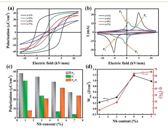
Fig. 8 (a) P-E loops of xNb ceramics and (b) corresponding I-E curves at room temperature. (c) The component dependent  $P_m$ ,  $P_r$  and  $\Delta P$  ( $P_m-P_r$ ). (d) The component dependent calculated energy storage density and efficiency.
