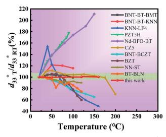
Fig. 7 Comparison of the temperature dependence of the  $d_{33}^{*}$  as normalized to the  $d_{33,\mathrm{RT}}^{*}$  for various systems.
