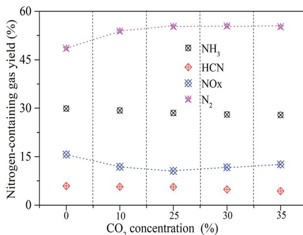
Fig. 9 The conversion ratio of nitrogen-containing gaseous products under different CO<sub>2</sub> concentrations.
