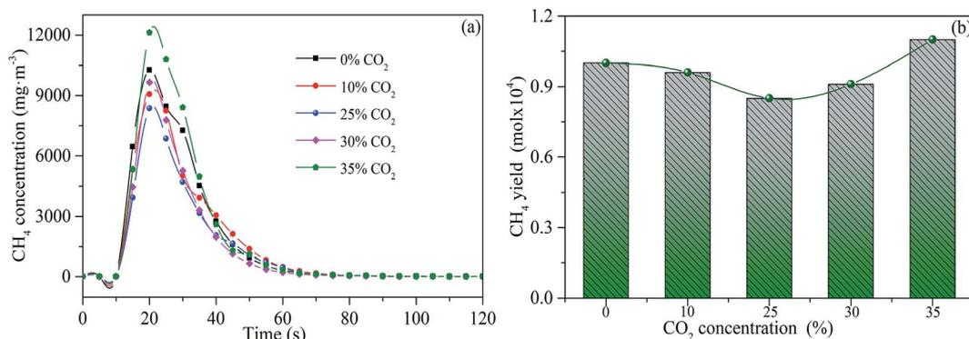
Fig. 7 Releasing rates (a) and yields (b) of CH<sub>4</sub> during sludge combustion under different CO<sub>2</sub> concentrations.
