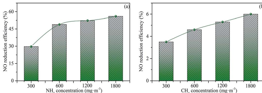
Fig. 14 Efficiency of NO reduction by  $\text{NH}_3$  (a) and  $\text{CH}_4$  (b). Reaction conditions:  $600 \text{ mg m}^{-3}$  of NO, 3 vol% of  $\text{O}_2$ , 25 vol% of  $\text{CO}_2$ , 3 vol% of  $\text{H}_2\text{O}$ , and balanced  $\text{N}_2$ , temperature =  $900 \text{ }^\circ\text{C}$ .
