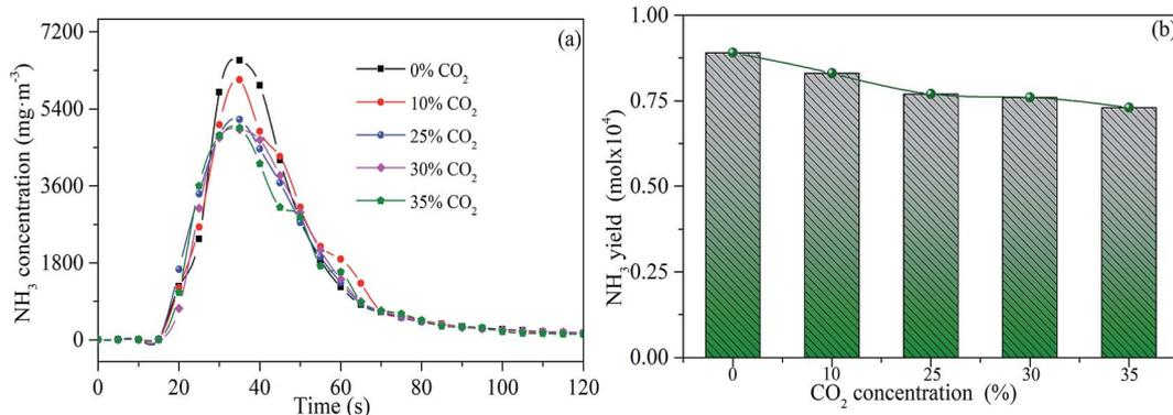
Fig. 8 Releasing rates (a) and yields (b) of NH<sub>3</sub> during sludge combustion under different CO<sub>2</sub> concentrations.
