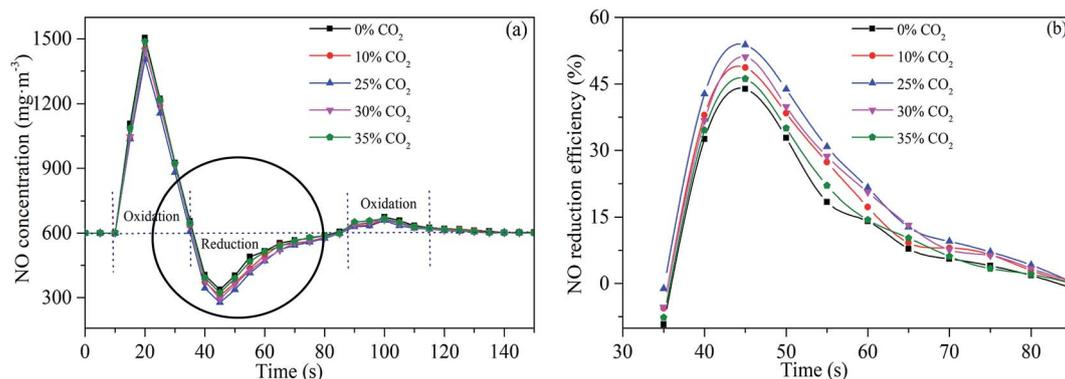
Fig. 10 Variation of NO concentration during NO reduction by sludge reburning (a) and the NO reduction efficiency (b) under different CO<sub>2</sub> concentrations. Reaction conditions: 600 mg m<sup>-3</sup> of NO, 200 mg m<sup>-3</sup> of SO<sub>2</sub>, 3 vol% of O<sub>2</sub>, and balanced N<sub>2</sub>, temperature = 900 °C.
