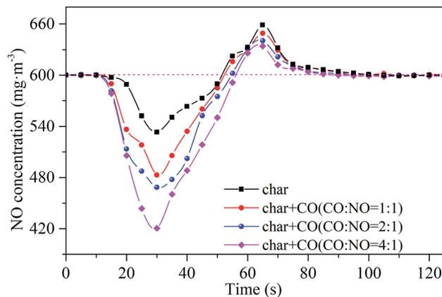
Fig. 13 Dynamic properties of NO reduction by CO in the presence of sludge char. Reaction conditions:  $600 \text{ mg m}^{-3}$  of NO, 25 vol% of  $\text{CO}_2$ , 3 vol% of  $\text{O}_2$ , and balanced  $\text{N}_2$ , temperature =  $900 \text{ }^\circ\text{C}$ .
