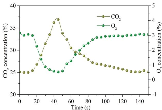
Fig. 11 Variation of O<sub>2</sub> and CO<sub>2</sub> concentrations during NO reduction by sludge reburning. Reaction conditions: 600 mg m<sup>-3</sup> of NO, 200 mg m<sup>-3</sup> of SO<sub>2</sub>, 25 vol% of CO<sub>2</sub>, 3 vol% of O<sub>2</sub>, and balanced N<sub>2</sub>, temperature = 900 °C.
