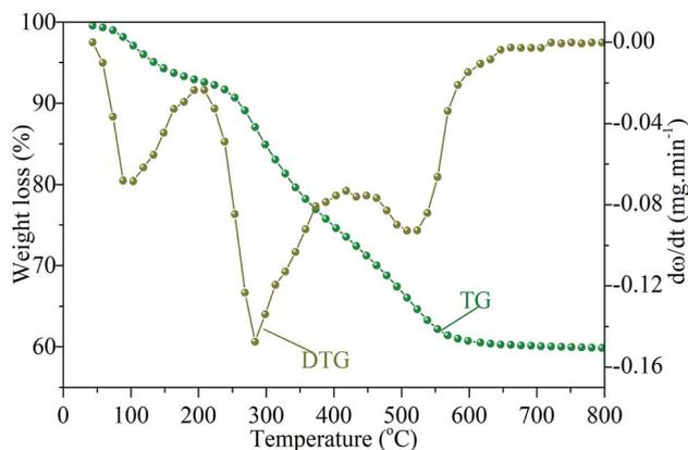
Fig. 2 TG and DTG results of sewage sludge with a heating rate of 20 K min<sup>-1</sup> under air atmosphere.
