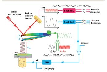
Fig. 1 Bimodal schematic description and control system. The two excitation frequencies are the first order flexural and torsional mode frequencies, respectively. The response of the cantilever contains two frequency components same as the excitation frequencies. The flexural signal is used for topography feedback and the flexural dissipation, while the torsional signal is utilized to detect the torsional dissipation.
