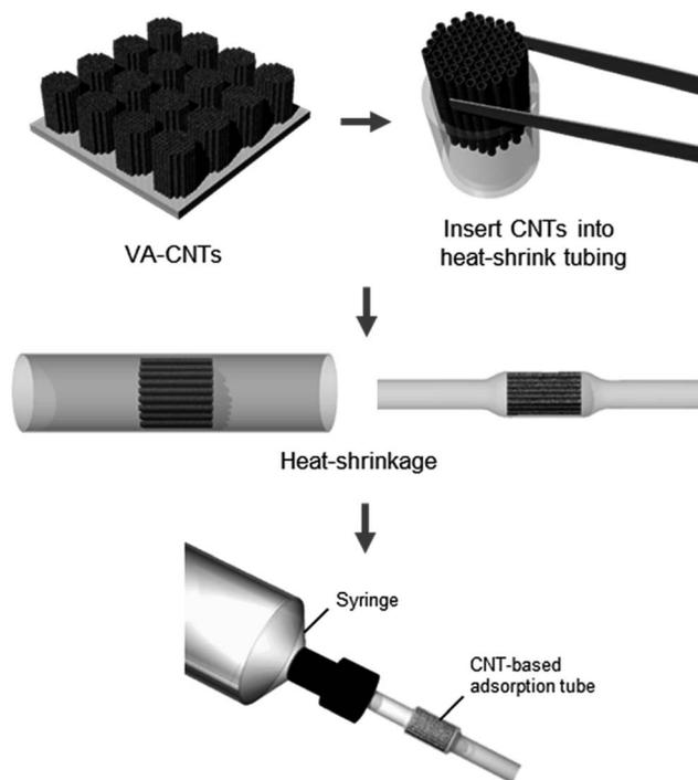
Fig. 1 Experimental scheme of fabricating CNT-based adsorption tube.
