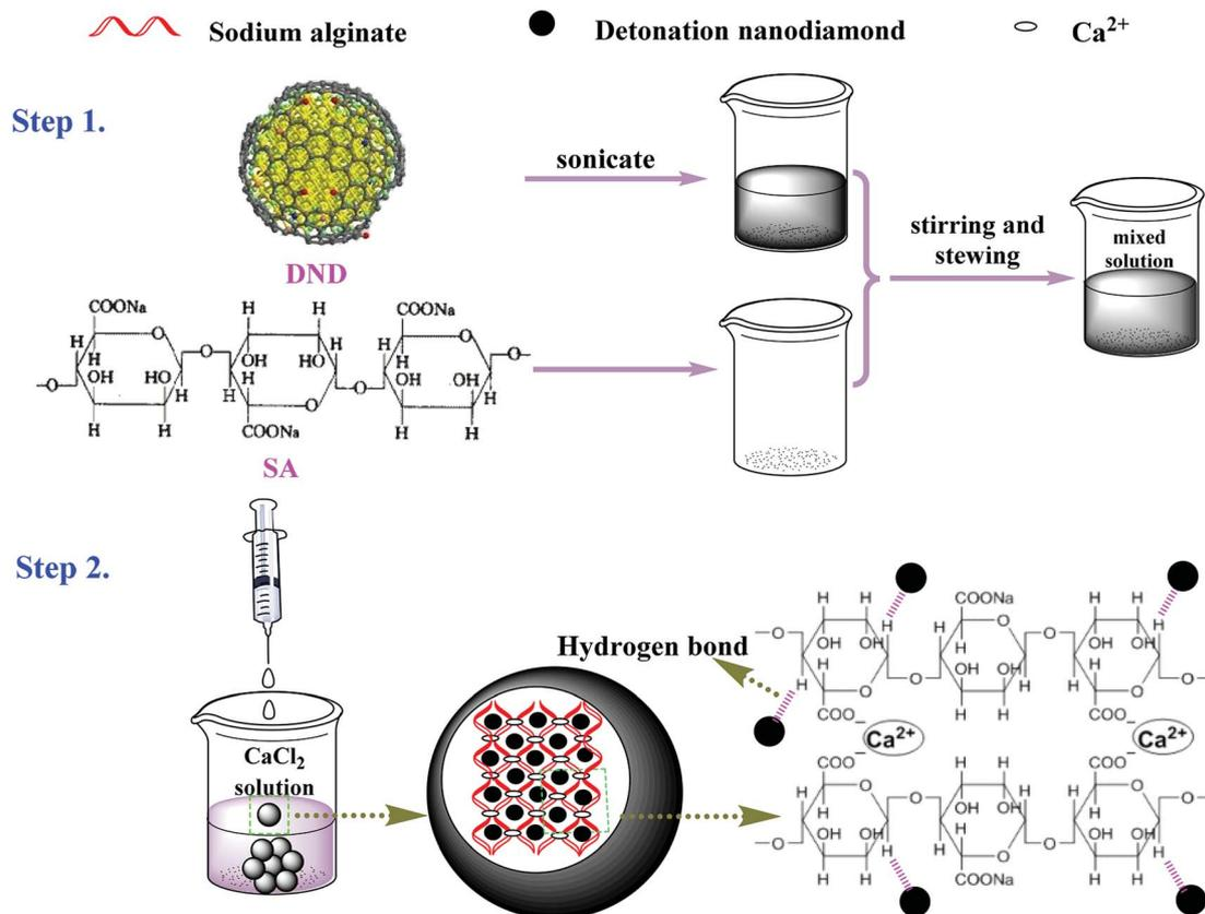
Scheme 1 Proposed mechanism for the formation of DND@SA hydrogel beads.
