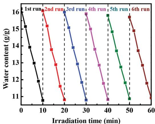
Fig. 6 Cycle test curves for sunlight-triggered water release of DND@SA hydrogel beads containing 0.8 mg mL<sup>-1</sup> DND. Each cycle consists of light irradiation for 10 min followed by a re-swelling process.
