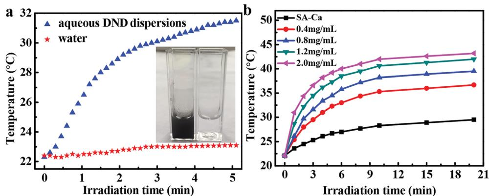
Fig. 3 (a) Temperature changes of pure water and 0.8 mg mL<sup>-1</sup> aqueous DND dispersions under irradiation with the sunlight of 100 mW cm<sup>-2</sup>. (Inset) Photograph of aqueous DND dispersions and distilled water after 5 min of irradiation. (b) Temperature changes of distilled water containing DND@SA hydrogel beads with different DND concentrations under irradiation with the sunlight of 100 mW cm<sup>-2</sup>.
