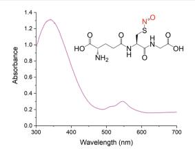
Fig. 7 DR UV-Vis spectrum of S-nitrosated emulsion with characteristic RSNO features. The structure of GSNO is shown as an inset.
