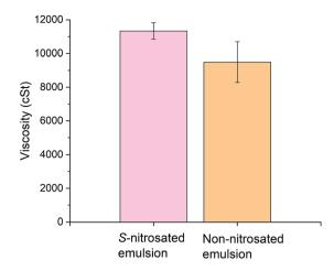
Fig. 2 Kinematic viscosity of S-nitrosated and non-nitrosated emulsion samples. All samples were tested in replicate ( $n \ge 3$ ) and the results are displayed as the mean  $\pm$  standard deviation.
