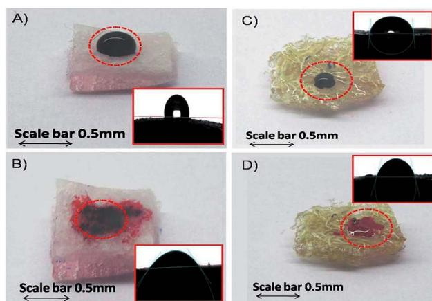
Fig. 5 Micrographs of different behaviour of water and oil droplets on the surfaces of (A and B) PDMS and (C and D) PDMS-*Luffa* sponges along with their corresponding contact angle images in the insets. Water forms a clear droplet on PDMS with contact angle of 112° (A) and PDMS-*Luffa* sponge with contact angle of 86° (B). The oil gets spread and absorbed on both PDMS with contact angle of 35° (C) and PDMS-*Luffa* sponge with contact angle of 68° (D).
