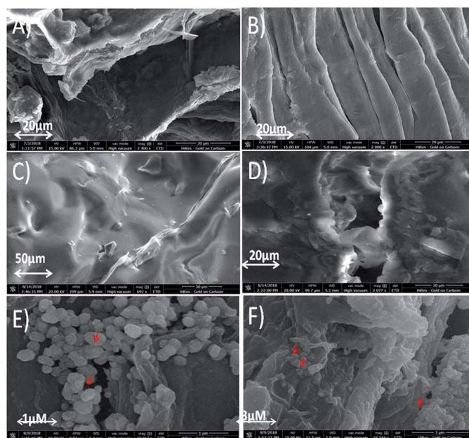
Fig. 4 SEM micrographs of (A) untreated *Luffa* fibre, (B) alkali treated *Luffa* fibre after 48 h, (C) PDMS sponge, (D) PDMS-*Luffa* sponge, (E and F) PDMS-*Luffa*-TiO<sub>2</sub> nanosponge.
