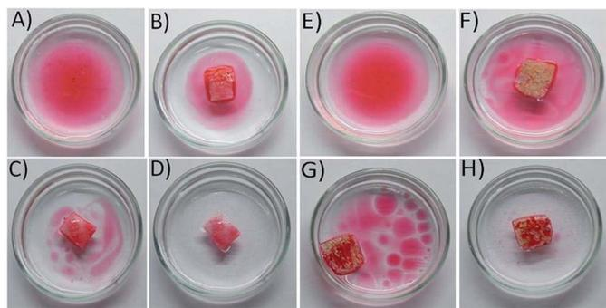
Fig. 7 Digital photographs showing the removal of oil from oil water mixture using PDMS sponge ((A)  $T_0 = 0$  s; (B)  $T_1 = 5$  s; (C)  $T_2 = 10$  s; (D)  $T_3 = 15$  s) and using PDMS-Luffa-TiO<sub>2</sub> nanosponge ((E)  $T_0 = 0$  s; (F)  $T_1 = 5$  s; (G)  $T_2 = 10$  s; (H)  $T_3 = 15$  s).
