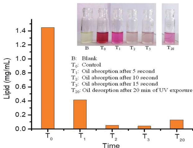
Fig. 8 Quantitative chart showing absorption and desorption of oil from oil water mixture by SPV method in PDMS-Luffa-TiO<sub>2</sub> nanosponge.
