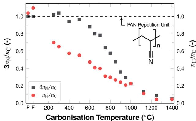
Fig. 4 Ratios of amounts of substance of nitrogen and carbon (grey) and hydrogen and carbon (red), relative to the ratio in the PAN repetition unit (black dashed line). P and F indicate PAN powder and PAN fibres, respectively.
