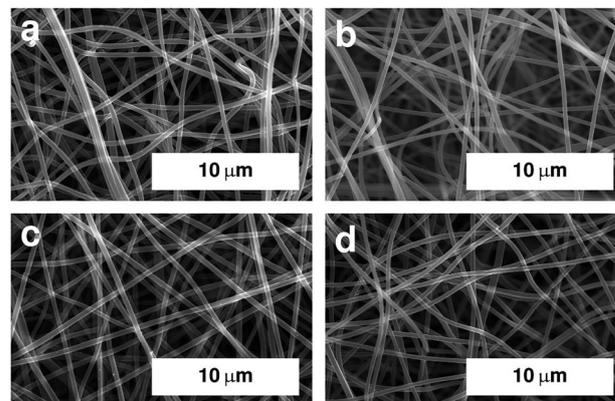
Fig. 1 SEM images of electrospun PAN fibres after stabilisation in air at 250 °C and carbonisation under argon at (a) 600 °C, (b) 800 °C, (c) 1000 °C, and (d) 1250 °C. Image for sample carbonised at 400 °C is shown in Fig. S1.†
