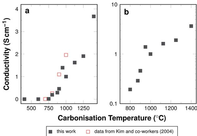
Fig. 9 (a) Calculated conductivity as a function of carbonisation temperature. Reference data from Kim and co-workers.<sup>42</sup> (b) Logarithmic plot of calculated conductivity as a function of carbonisation temperature in a selected range.
