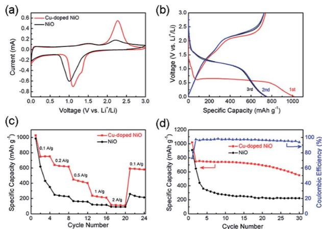
Fig. 5 (a) CV curves of Cu-doped NiO and original NiO at 0.1 mV s<sup>-1</sup> scan rate, (b) galvanostatic charge–discharge (GCD) profiles for first three cycles of Cu-doped NiO at 100 mA g<sup>-1</sup>, (c) rate capability and (d) cycling performances for NiO and Cu-doped NiO.
