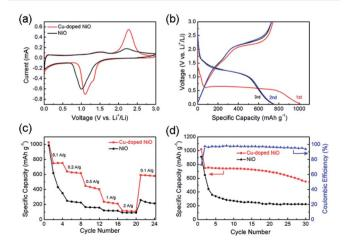
Fig. 5 (a) CV curves of Cu-doped NiO and original NiO at  $0.1 \, \text{mV s}^{-1}$  scan rate, (b) galvanostatic charge–discharge (GCD) profiles for first three cycles of Cu-doped NiO at 100 mA  $g^{-1}$ , (c) rate capability and (d) cycling performances for NiO and Cu-doped NiO.
