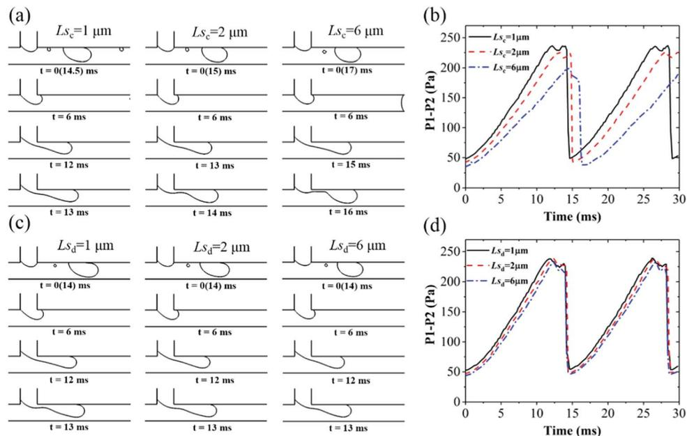
Fig. 8 Dropping regime with  $Q_d = 0.2 \text{ mL h}^{-1}$  and  $Q_c = 2 \text{ mL h}^{-1}$ . (a) Droplet generation process and (b) pressure drop through the thread with time under different  $L_{s_c}$  with  $L_{s_d} = 0.5 \mu\text{m}$ . (c) Droplet generation process and (d) pressure drop through the thread with time under different  $L_{s_d}$  with  $L_{s_c} = 0.5 \mu\text{m}$ .
