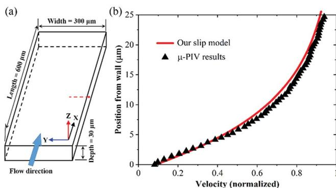
Fig. 4 (a) Geometry of the microchannel for slip model validation. (b) Velocity profiles from experiment and simulation along the line of  $x = 300 \mu\text{m}$  and  $z = 15 \mu\text{m}$ ; the  $x$ -axis is the velocity normalized by the free stream velocity and the  $y$ -axis is the distance from the wall.
