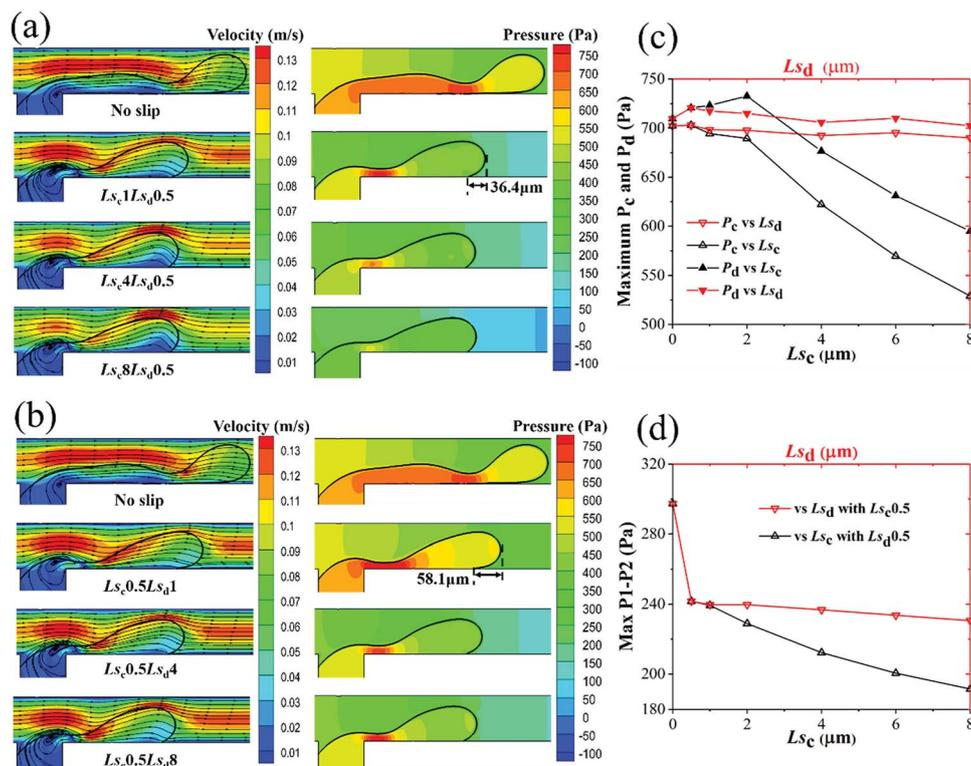
Fig. 10 Velocity contours with streamlines and pressure contours of (a) different  $L_{sc}$  with  $L_{sd} = 0.5 \mu\text{m}$  and (b) different  $L_{sd}$  with  $L_{sc} = 0.5 \mu\text{m}$ . (c) Maximum pressure at continuous and dispersed phase inlets and (d) maximum pressure drop across the thread as functions of  $L_{sc}$  and  $L_{sd}$  in a dripping regime with  $Q_d = 0.2 \text{ mL h}^{-1}$  and  $Q_c = 2 \text{ mL h}^{-1}$ .
