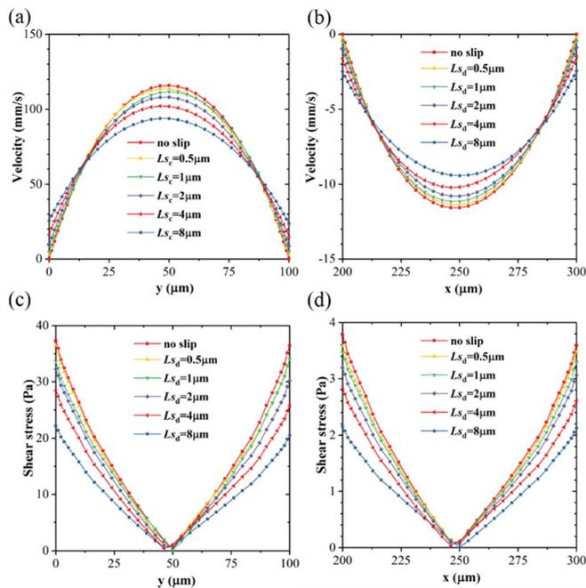
Fig. 6 Velocity distribution at (a) line  $x = 150 \mu\text{m}$  along  $y$ -direction and (b) line  $y = 200 \mu\text{m}$  along the  $x$ -direction on the symmetry plane for different  $L_{s_c}$  and  $L_{s_d}$  with  $Q_d = 0.2 \text{ mL h}^{-1}$  and  $Q_c = 2 \text{ mL h}^{-1}$ ; (c) and (d) represent resistant shear stresses exerted by the slow object (adjacent fluid or wall) corresponding to (a) and (b).
