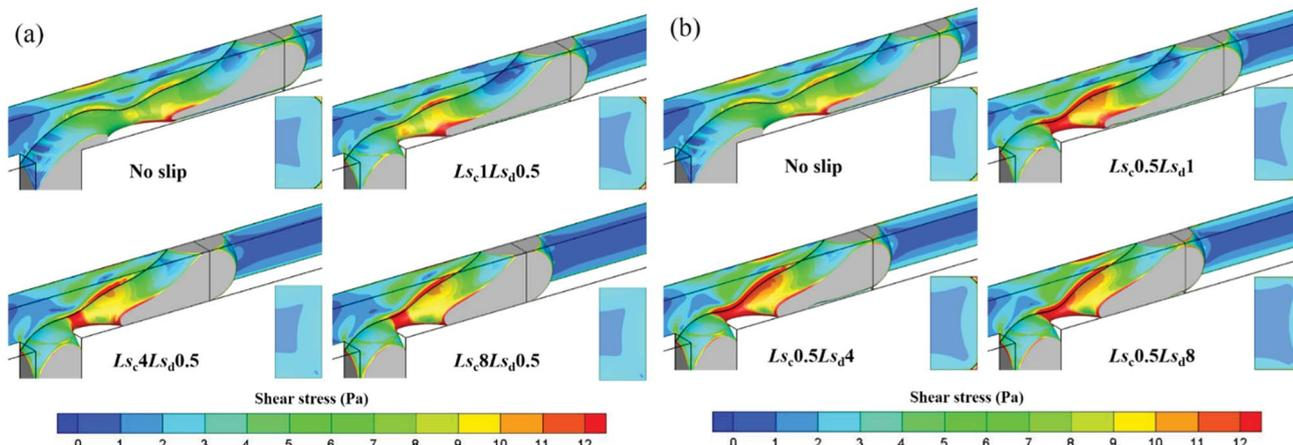
Fig. 13 Droplet surface colored by shear stress magnitude with (a) different  $L_{sc}$  when  $L_{sd} = 0.5 \mu\text{m}$  and (b) different  $L_{sd}$  when  $L_{sc} = 0.5 \mu\text{m}$  for  $Q_d = 0.09 \text{ mL h}^{-1}$  and  $Q_c = 0.18 \text{ mL h}^{-1}$  in a squeezing regime.
