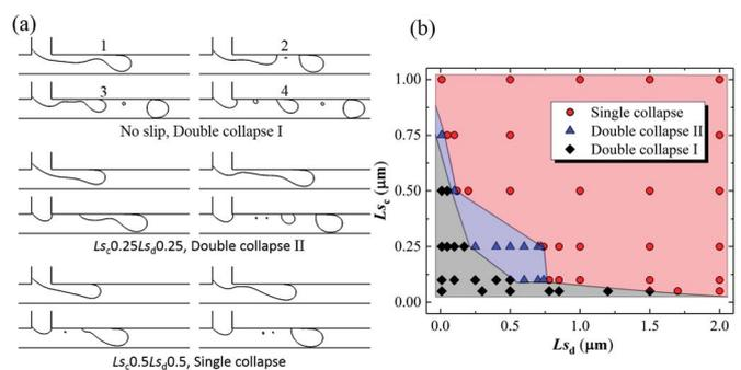
Fig. 16 (a) Three different droplet generation states and (b) phase diagram of droplet generation state as a function of  $L_{sc}$  and  $L_{sd}$  in a dripping regime with  $Q_d = 0.2 \text{ mL h}^{-1}$  and  $Q_c = 2 \text{ mL h}^{-1}$ .
