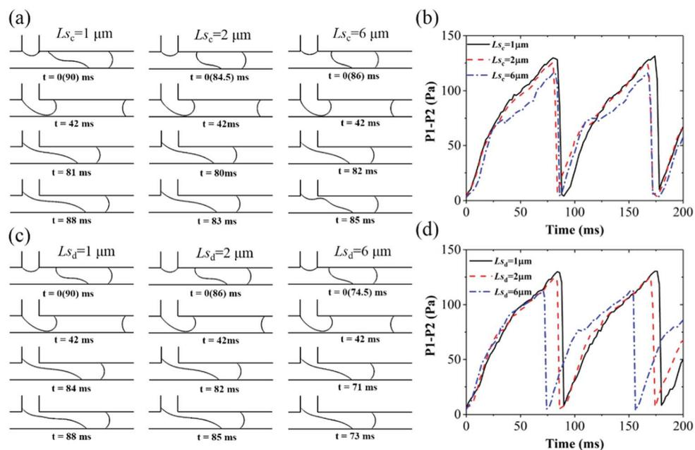
Fig. 9 Squeezing regime with  $Q_d = 0.09 \text{ mL h}^{-1}$  and  $Q_c = 0.18 \text{ mL h}^{-1}$ . (a) Droplet generation process and (b) pressure drop through the thread with time under different  $L_{s_c}$  with  $L_{s_d} = 0.5 \mu\text{m}$ . (c) Droplet generation process and (d) pressure drop through the thread with time under different  $L_{s_d}$  with  $L_{s_c} = 0.5 \mu\text{m}$ .
