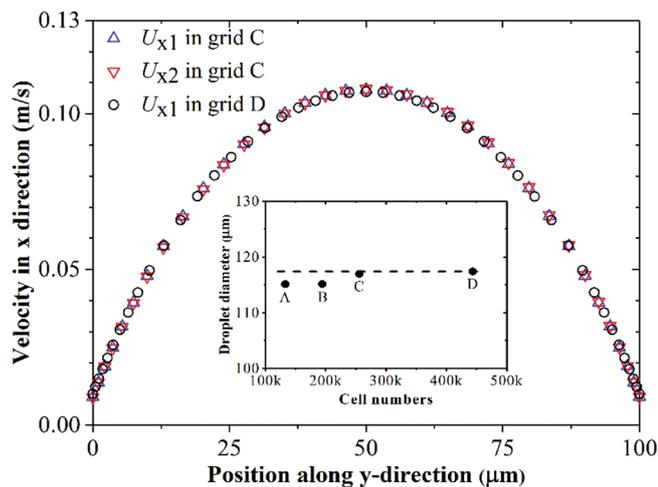
Fig. 3 Grid independence study for  $Q_d = 0.2 \text{ mL h}^{-1}$  and  $Q_c = 2 \text{ mL h}^{-1}$  with moderate slip lengths of  $2 \mu\text{m}$ .  $U_{x1}$  and  $U_{x2}$  represent the  $x$ -velocity along the  $y$ -direction at  $x = 100 \mu\text{m}$  and  $x = 150 \mu\text{m}$  on the symmetry plane, respectively.
