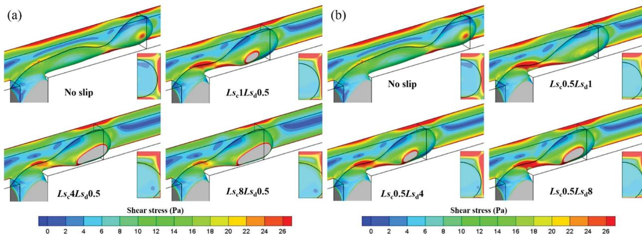
Fig. 12 Droplet surface colored by shear stress magnitude with (a) different  $L_{sc}$  when  $L_{sd} = 0.5 \mu\text{m}$  and (b) different  $L_{sd}$  when  $L_{sc} = 0.5 \mu\text{m}$  for  $Q_d = 0.2 \text{ mL h}^{-1}$  and  $Q_c = 2 \text{ mL h}^{-1}$  in a dripping regime.
