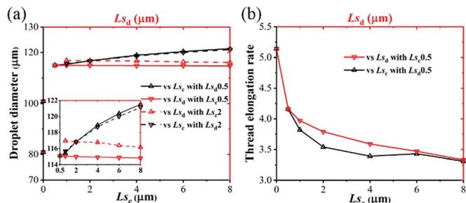
Fig. 14 (a) Droplet diameter and (b) thread elongation rate as functions of  $L_{sc}$  and  $L_{sd}$  in a dripping regime with  $Q_d = 0.2 \text{ mL h}^{-1}$  and  $Q_c = 2 \text{ mL h}^{-1}$ .
