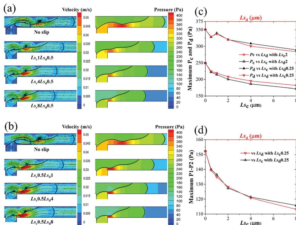
Fig. 11 Velocity contours with streamlines and pressure contours of (a) different  $L_{sc}$  when  $L_{sd} = 0.5 \mu\text{m}$  and (b) different  $L_{sd}$  when  $L_{sc} = 0.5 \mu\text{m}$ . (c) Maximum pressure on continuous and dispersed phase inlets and (d) maximum pressure drop across the thread as functions of  $L_{sc}$  and  $L_{sd}$  in dripping regime with  $Q_d = 0.09 \text{ mL h}^{-1}$  and  $Q_c = 0.18 \text{ mL h}^{-1}$ .
