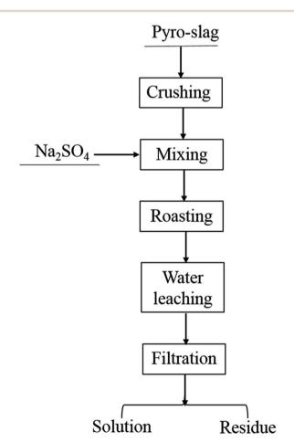
Fig. 4 Flow sheet for the roasting-leaching process
