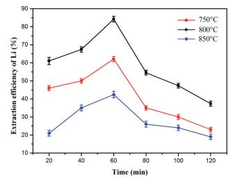
Fig. 8 Effect of roasting time on leaching efficiency of lithium at different roasting temperatures ( $Na_2So_4/Li$  molar ratio of 3 : 1).
