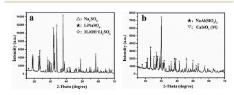
Fig. 12 XRD patterns of the leaching solution (a) and leached residue (b).
