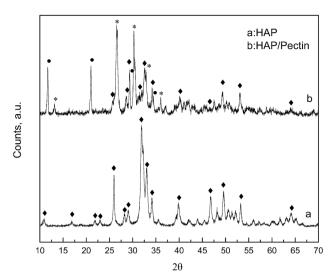
Fig. 2 XRD patterns of HAP and optimized HAP/pectin hybrid. Principal diffractions of HAP (♠); CaPO<sub>3</sub>(OH)·2H<sub>2</sub>O (♠); CaPO<sub>3</sub>(OH) (\*).
