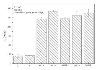
Fig. 1 HAP/pectin hybrid materials compared to precursor materials, when  $0.5 \, \mathrm{g} \, \mathrm{L}^{-1}$  of adsorbents were used to treat 180 mg  $\mathrm{L}^{-1} \, \mathrm{Zn}^{2+}$  at pH 5.0. The mass ratio of each sample is provided, 6H1P used 6 grams of HAP and 1 gram of pectin (\*denotes there was no pretreatment by ethanol before drying).
