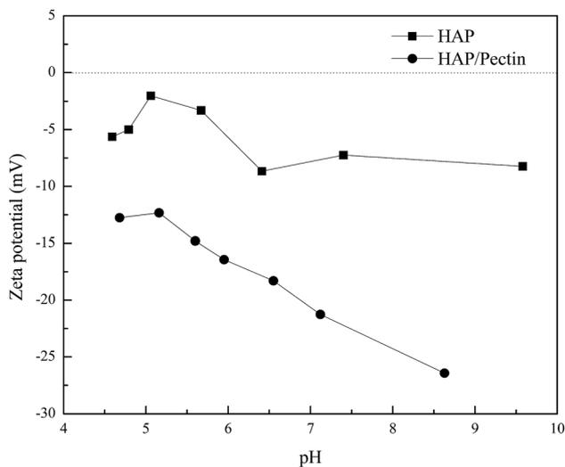
Fig. 8 Zeta potential for HAP and HAP/pectin hybrid suspended in 1 mM KNO<sub>3</sub>.
