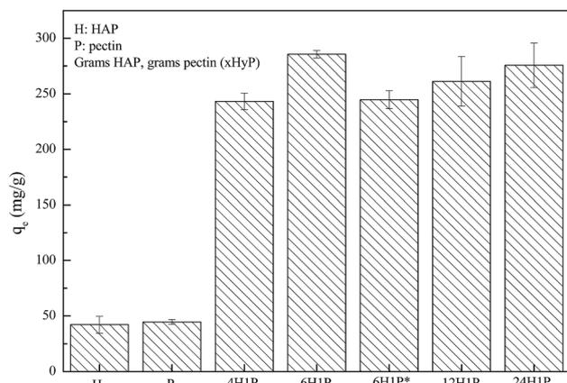
Fig. 1 HAP/pectin hybrid materials compared to precursor materials, when  $0.5 \text{ g L}^{-1}$  of adsorbents were used to treat  $180 \text{ mg L}^{-1} Zn^{2+}$  at pH 5.0. The mass ratio of each sample is provided, 6H1P used 6 grams of HAP and 1 gram of pectin (\*denotes there was no pretreatment by ethanol before drying).
