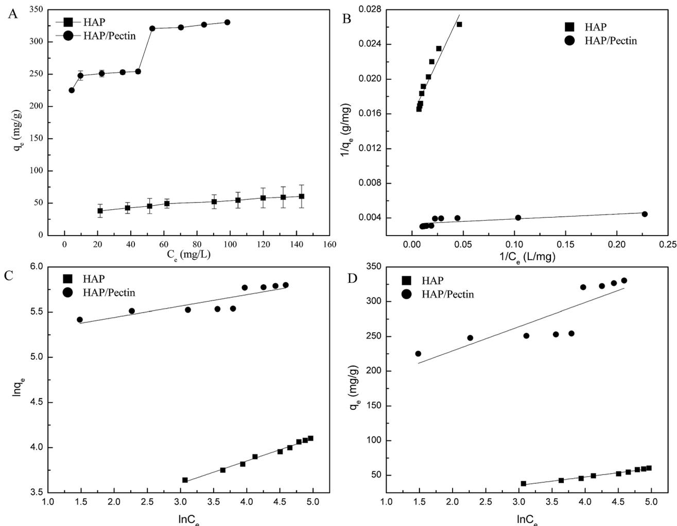
Fig. 6 Sorption isotherms of  $Zn^{2+}$  onto HAP and HAP/pectin. (A) The equilibrium sorption  $q_e$  as a function of the equilibrium  $C_e$ ; (B) the Langmuir model analysis; (C) the Freundlich model analysis; (D) Temkin model analysis.
