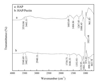
Fig. 3 FTIR spectrum of HAP and HAP/pectin hybrid.
