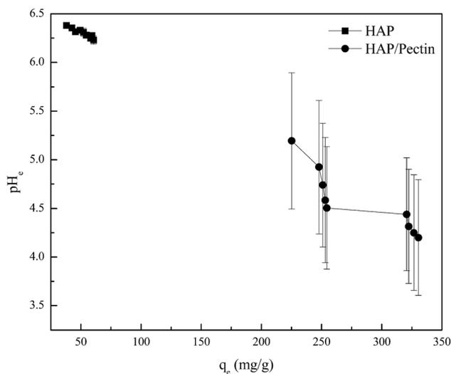
Fig. 7 The equilibrium pH ( $pH_e$ ) vs. the corresponding equilibrium zinc sorption capacity ( $q_e$ ). The  $pH_e$  data was collected simultaneously during the isotherm tests shown in Fig. 6.
