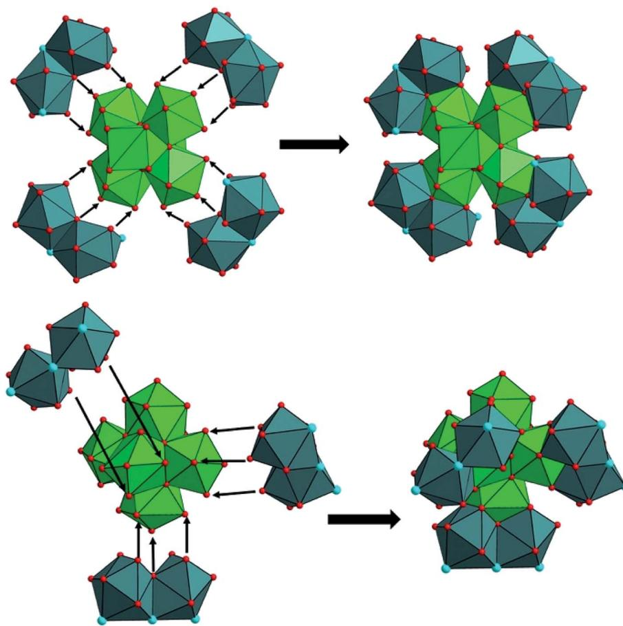
Fig. 7 Different connection manners between the central hexanuclear core  $[U_6O_4(OH)_4]$  and peripheral dinuclear uranium sub-units to form different uranium clusters (top;  $\{U_{14}\}$ , bottom;  $\{U_{12}\}$ <sup>39</sup>).
