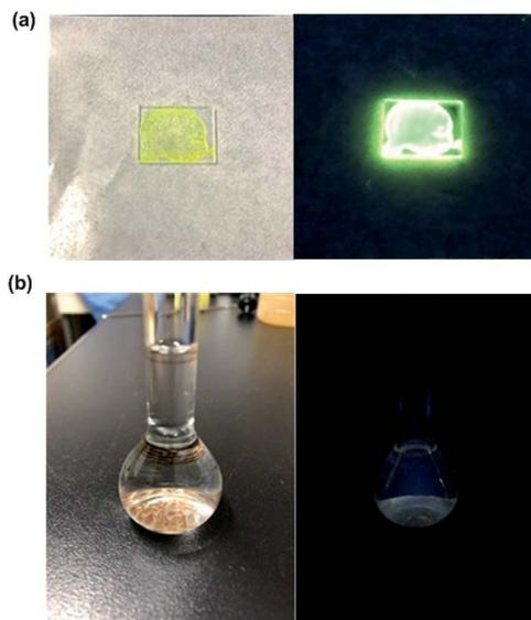
Fig. 6 (a) PolyBP5 film under ambient light (left) and under exposure to a UV lamp ( $\lambda_{ex} = 365$  nm) (right). (b) PolyBP5 in THF solution under ambient light (left) and under exposure to a UV lamp ( $\lambda_{ex} = 365$  nm) (right).
