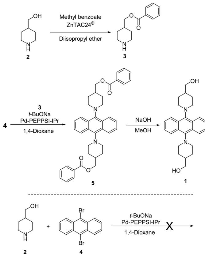
Scheme 1 Synthesis of AIE-active monomer 9,10-bis(4-hydroxymethyl)piperidylanthracene (**1**).
