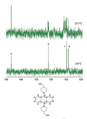
Fig. 1 Magnified view of the aromatic region of the  $^{13}$ C NMR (125 MHz, DMSO- $d_6$ ) spectrum of 1 at 20.5 °C (top) and 140 °C (bottom).
