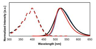
Fig. 5 Absorption and fluorescence spectra of 1 and BPA. Solid fluorescence of 1 (blue), as well as solution fluorescence of 1 (black) and BPA (red) (dashed lines: absorption spectra; solid lines: fluorescence spectra). The intensities of the spectra were normalized. All spectra were measured in THF solution ( $10^{-4}$  M).
