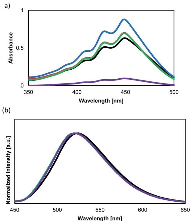
Fig. 4 (a) Absorption spectra of monomer **1** (black), as well as copolymers PolyBP5 (red), PolyBP10 (green), PolyBP20 (blue), and PolyBHMPA (purple). All spectra were measured in THF ( $10^{-4}$  M). (b) Fluorescence spectra of monomer **1** (black), as well as copolymers PolyBP5 (red), PolyBP10 (green), PolyBP20 (blue), and PolyBHMPA (purple). All spectra were measured in THF ( $10^{-4}$  M).
