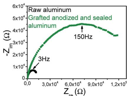
Fig. 5 Nyquist diagrams in 0.1 M KCl under O.C.P. conditions for raw aluminium (black line) and aluminium grafted with 4-nitrobenzenediazonium anodized and sealed (green line).
