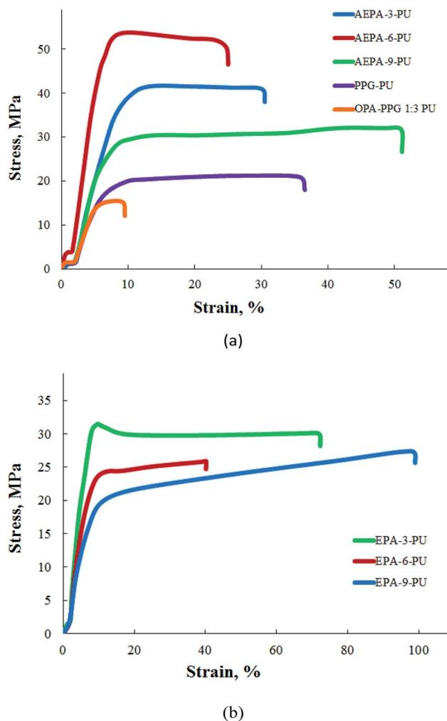
Fig. 10 Tensile tests of polymers.
