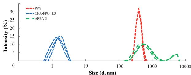
Fig. 1 Particle size distribution in the environment of toluene, determined by dynamic light scattering.
