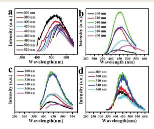
Fig. 3 The fluorescence emission spectra of GQDs-3/yellow samples with excitation wavelengths from 360 nm to 520 nm (a), GQDs-4/green with excitation wavelengths from 300 nm to 400 nm (b), GQDs-5/cyan with excitation wavelengths from 280 nm to 380 nm (c), and GQDs-6/light blue samples with excitation wavelengths from 280 nm to 360 nm (d).
