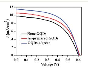
cells 4 J-V characteristics of the solar based P3HT:PCBM:GQDs active layers with different GQDs
