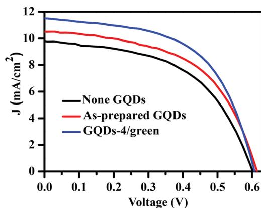
Fig. 4 *J*–*V* characteristics of the solar cells based on P3HT:PCBM:GQDs active layers with different GQDs.
