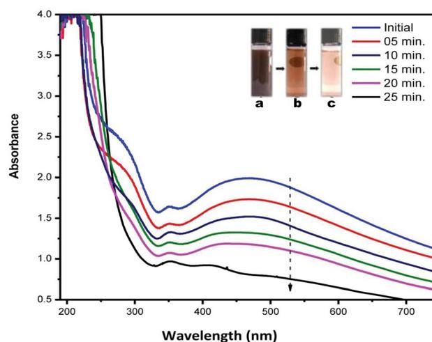
Fig. 7 UV-visible absorbance spectra of AC-AgNPs solution recorded at different time interval after the addition of H<sub>2</sub>O<sub>2</sub> (inset: reacting solution (a) initial (b) after 15 min (c) after 25 min).
