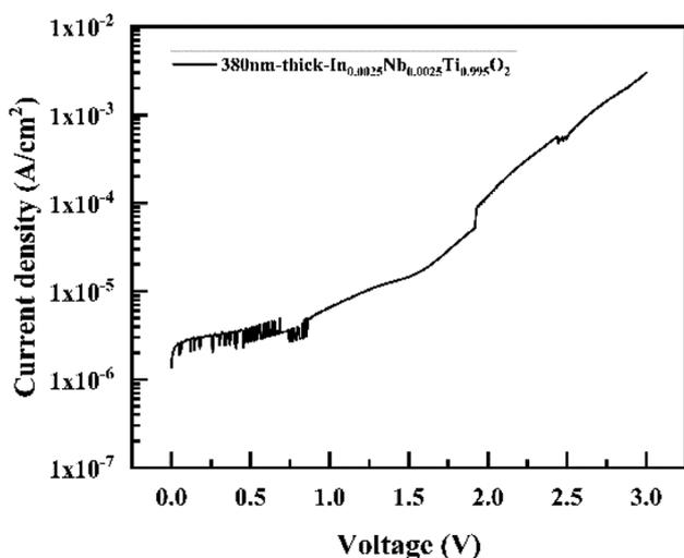
Fig. 9 The leakage current density versus voltage curve of the ITO/In<sub>0.0025</sub>Nb<sub>0.0025</sub>Ti<sub>0.995</sub>O<sub>2</sub>/ITO capacitor annealed at 400 °C for 30 minutes.
