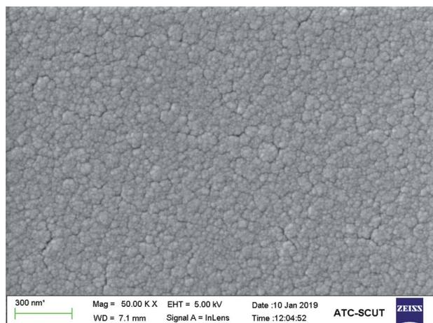
Fig. 3 SEM image of the  $\text{In}_{0.0025}\text{Nb}_{0.0025}\text{Ti}_{0.995}\text{O}_2$  film on ITO/glass substrates annealed at  $400 \text{ }^\circ\text{C}$  for 30 minutes.
