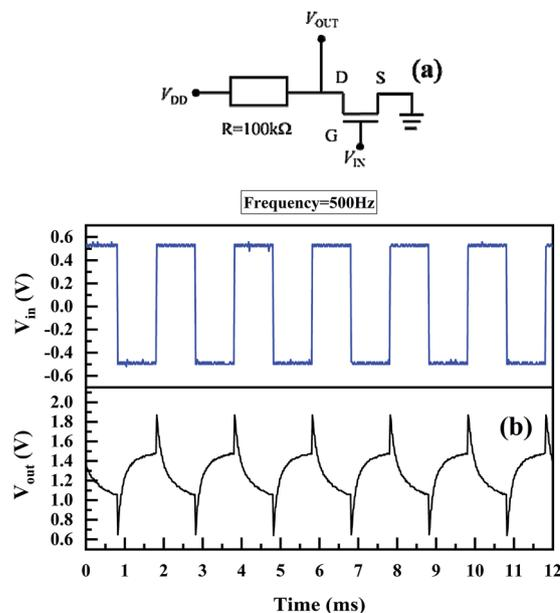
Fig. 8 (a) The circuit of the inverter; (b) the input and output voltage of a resistor-loaded inverter with an  $\text{In}_{0.0025}\text{Nb}_{0.0025}\text{Ti}_{0.995}\text{O}_2$ /IZO TFT and a resistor (100 k $\Omega$ ) at 500 Hz ( $V_{\text{DD}} = 1.8 \text{ V}$ ).
