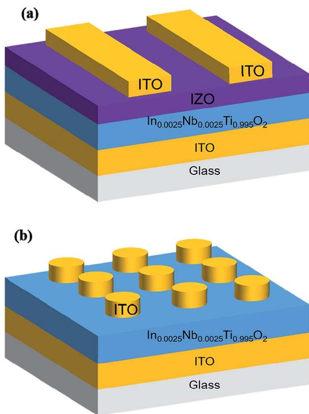
Fig. 1 Schematic structures of (a) the TFT with  $\text{In}_{0.0025}\text{Nb}_{0.0025}\text{Ti}_{0.995}\text{O}_2$  gate insulator and (b) the capacitors with ITO/ $\text{In}_{0.0025}\text{Nb}_{0.0025}\text{Ti}_{0.995}\text{O}_2$ /ITO stacks.
