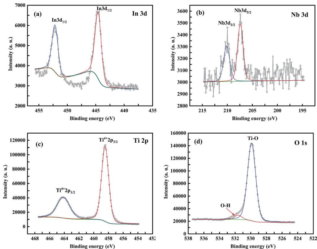
Fig. 6 XPS spectra of the  $\text{In}_{0.0025}\text{Nb}_{0.0025}\text{Ti}_{0.995}\text{O}_2$  films on ITO/glass substrates annealed at  $400^\circ\text{C}$  for 30 minutes, including: (a) In 3d, (b) Nb 3d, (c) Ti 2p, (d) O 1s.
