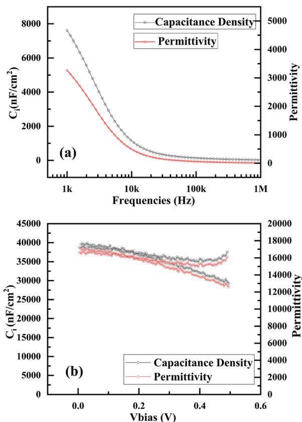
Fig. 7 (a) The frequency dependences of capacitance density (black curve) and permittivity (red curve), (b) the quasi-static  $C_i$ – $V$  curve of the capacitor with the ITO/ $\text{In}_{0.0025}\text{Nb}_{0.0025}\text{Ti}_{0.995}\text{O}_2$ /ITO structure annealed at 400 °C for 30 minutes.
