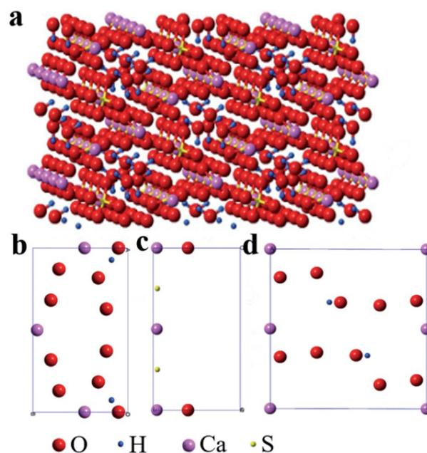
Fig. 6 Molecular model of the obtained rod-shaped  $\alpha$ - $\text{CaSO}_4 \cdot 0.5\text{H}_2\text{O}$  crystals (a) 3D model ( $2 \times 2 \times 2$  supercell) along the  $c$ -axis direction and (b–d) facet slice models: (b) (001) and (002), (c) (200) and (400), (d) (020).
