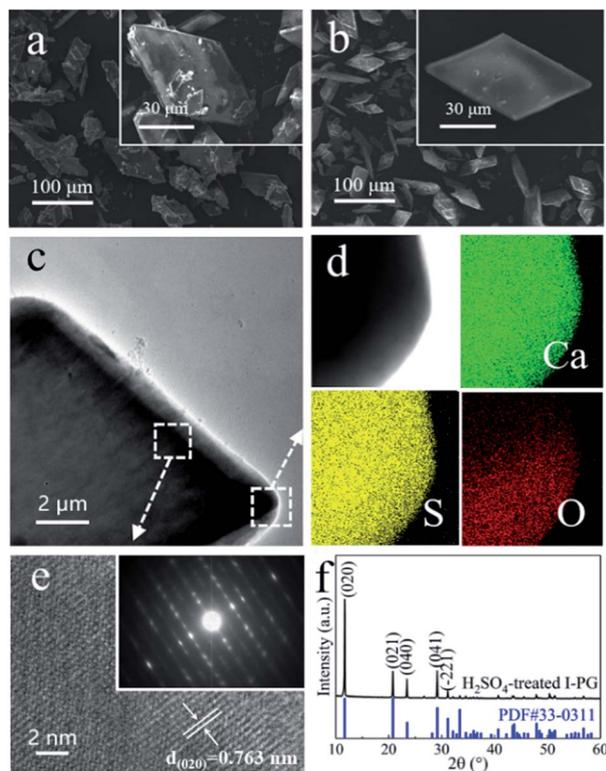
Fig. 1 (a) SEM image of I-PG; (b) SEM and (c) TEM images of the  $\text{H}_2\text{SO}_4$ -treated I-PG, and (d) the corresponding elemental mapping images showing the distribution of Ca, S and O; (e) HRTEM and SAED (inset) images and (f) XRD pattern of the  $\text{H}_2\text{SO}_4$ -treated I-PG.
