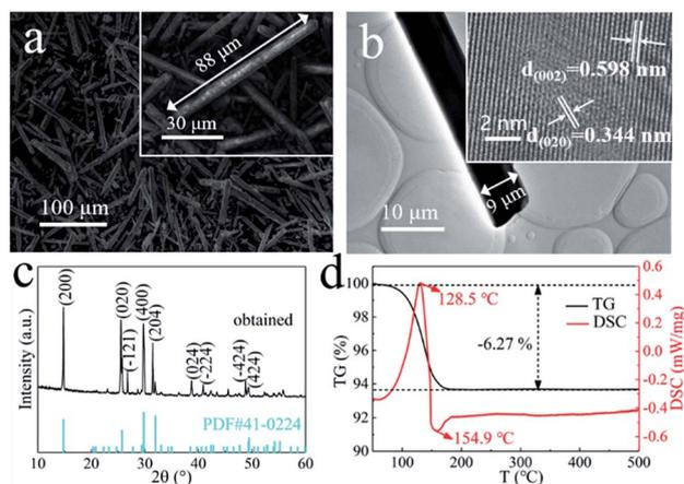
Fig. 2 (a) SEM and (b) TEM images of the  $\alpha\text{-CaSO}_4 \cdot 0.5\text{H}_2\text{O}$  crystals prepared in 50 mM PT aqueous solution for 6 h; (c) XRD pattern and (d) TG-DSC analysis of the obtained  $\alpha\text{-CaSO}_4 \cdot 0.5\text{H}_2\text{O}$  crystals. The inset images in (b) show the corresponding HRTEM image of obtained crystal.
