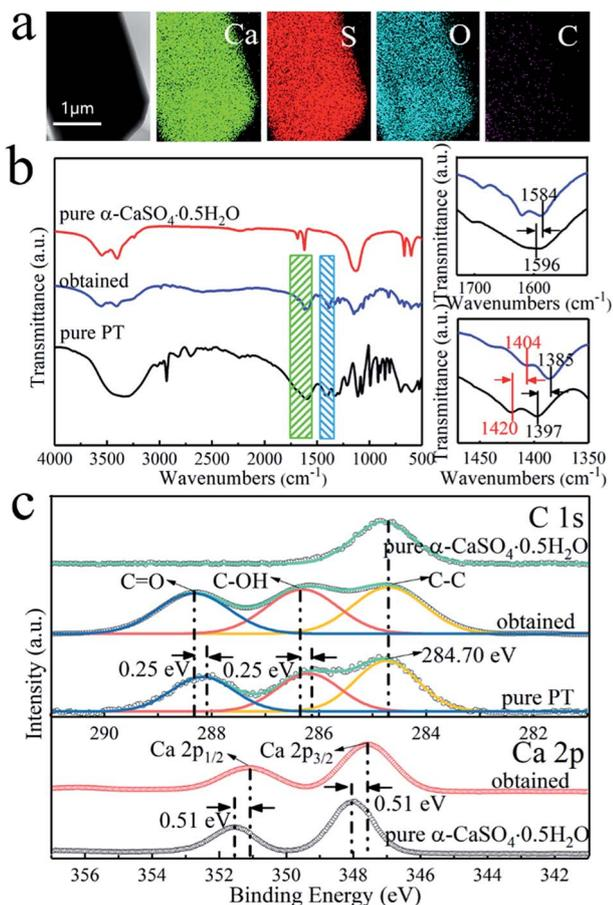
Fig. 5 (a) Elemental mapping images of the obtained rod-shaped  $\alpha$ - $\text{CaSO}_4 \cdot 0.5\text{H}_2\text{O}$  crystals prepared in 50 mM PT aqueous solution; (b) FT-IR spectra of PT, pure  $\alpha$ - $\text{CaSO}_4 \cdot 0.5\text{H}_2\text{O}$  crystals and the obtained crystals; (c) C 1s and Ca 2p XPS spectra of PT, pure  $\alpha$ - $\text{CaSO}_4 \cdot 0.5\text{H}_2\text{O}$  and obtained crystals.
