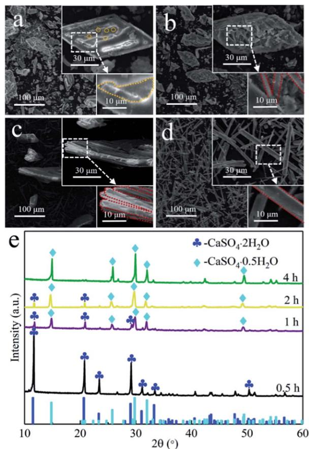
Fig. 3 SEM images of the intermediates of rod-shaped  $\alpha$ - $\text{CaSO}_4 \cdot 0.5\text{H}_2\text{O}$  crystals intermediates obtained after proceeding the reaction for (a) 0.5, (b) 1, (c) 2, and (d) 4 h; (e) XRD patterns of corresponding intermediates.
