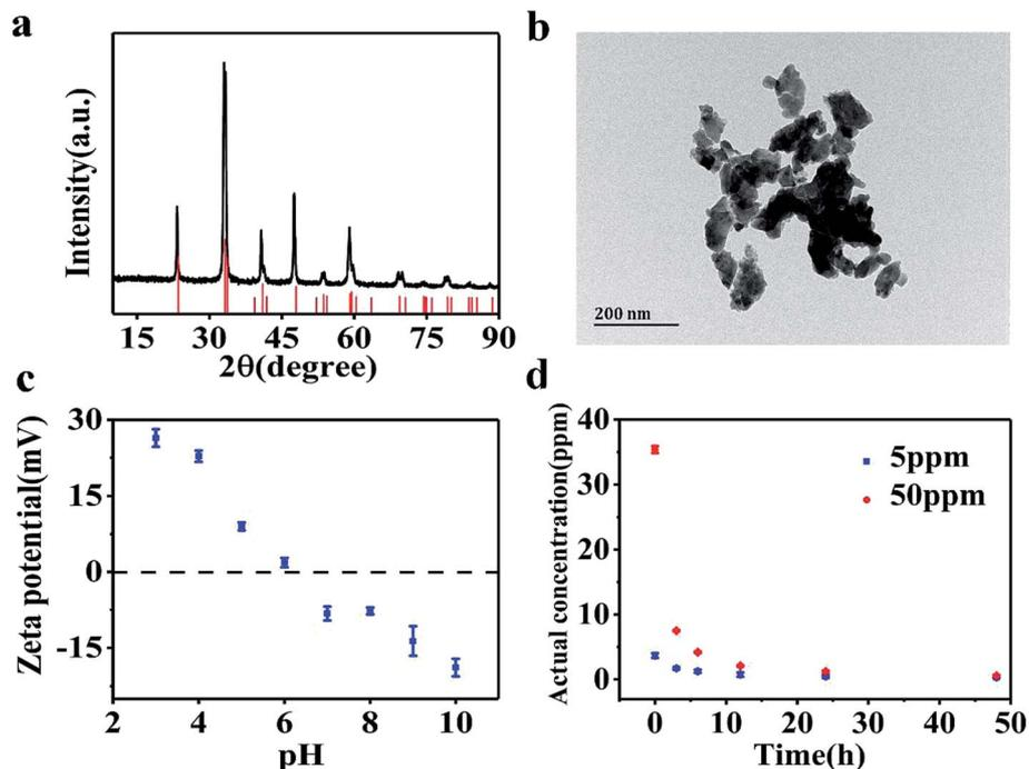
Fig. 1 (a) XRD pattern of LaCoO<sub>3</sub> NPs. (b) TEM image of LaCoO<sub>3</sub> NPs. (c) Zeta potential of LaCoO<sub>3</sub> NPs as a function of pH. (d) Actual concentration of LaCoO<sub>3</sub> NPs in suspension.
