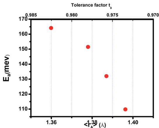
Fig. 7 Activation energy vs. the tolerance factor  $t_g$  and the average ionic radius of the A-site  $\langle r_A \rangle$  for  $(\text{La}_{1-x}\text{Pr}_x)_{0.67}\text{Ba}_{0.33}\text{MnO}_3$  ( $0 \leq x \leq 0.30$ ).
