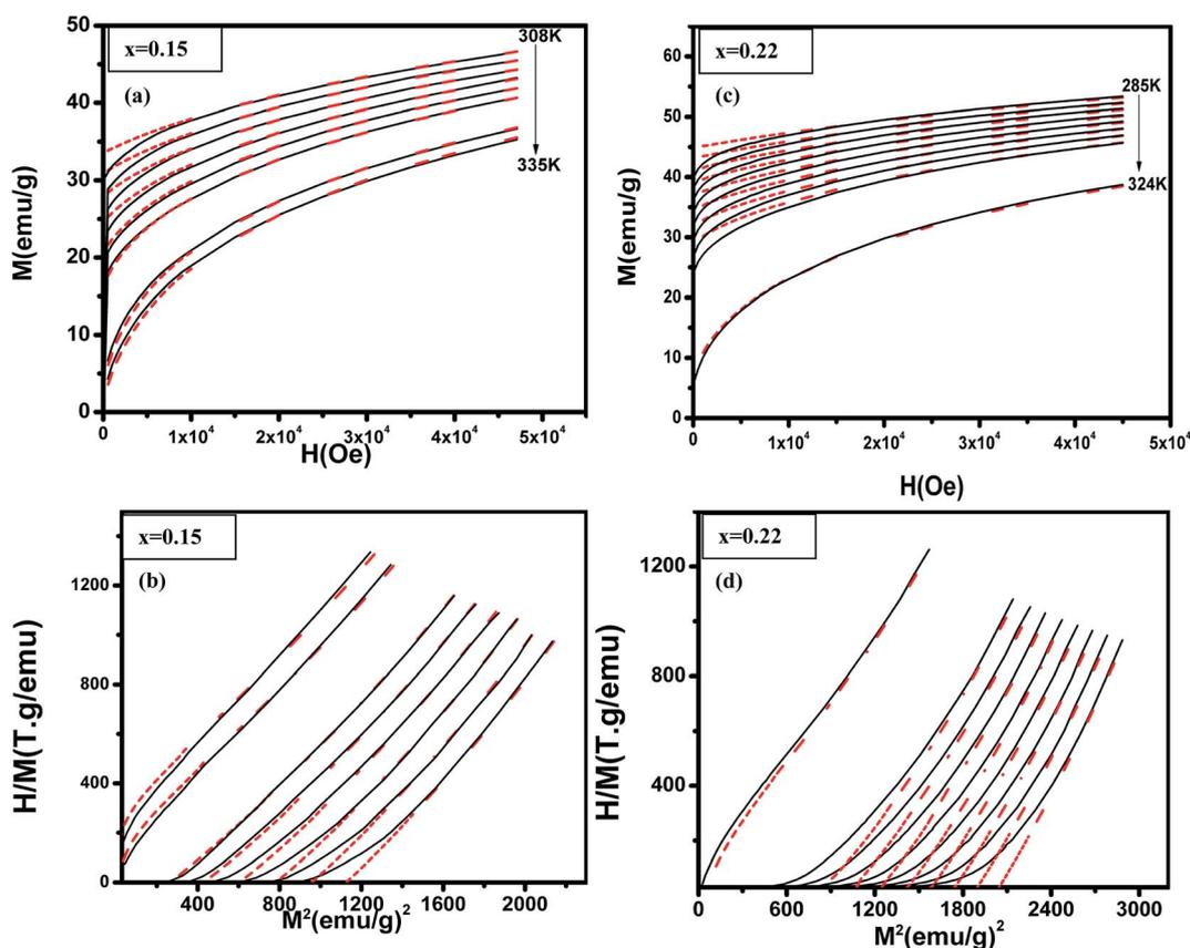
**Fig. 5**  $(\text{La}_{1-x}\text{Pr}_x)_{0.67}\text{Ba}_{0.33}\text{MnO}_3$  ( $x = 0.10$  and  $x = 0.15$ ) experimental (black lines) and simulated (red dots) curves showing ((a) and (c)) magnetization as a function of applied magnetic field, at the indicated temperature values and ((b) and (d)) corresponding  $H/M$  vs.  $M^2$  Arrott plots.
