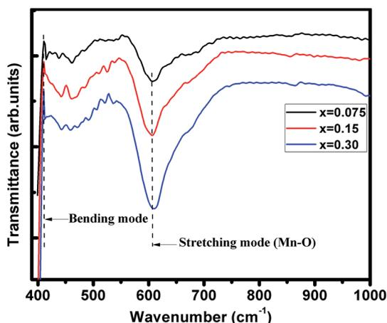
Fig. 2 Infrared phonon spectra of ( $x = 0.075, 0.15$  and  $0.30$ ) samples.
