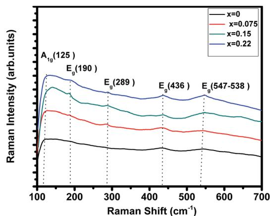
Fig. 3 Raman spectrum of  $(\text{La}_{1-x}\text{Pr}_x)_{0.67}\text{Ba}_{0.33}\text{MnO}_3$  ( $x = 0, 0.075, 0.15$  and  $x = 0.22$ ) samples.
