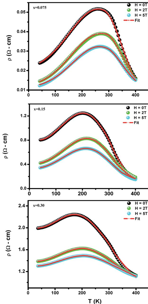
Fig. 6 Temperature dependence of the resistivity  $\rho(T, H)$  at without and with different applied magnetic fields for  $(\text{La}_{1-x}\text{Pr}_x)_{0.67}\text{Ba}_{0.33}\text{MnO}_3$  with  $x = 0.075, 0.15$  and  $x = 0.30$ . Red solid line corresponds to fit by eqn (9).
