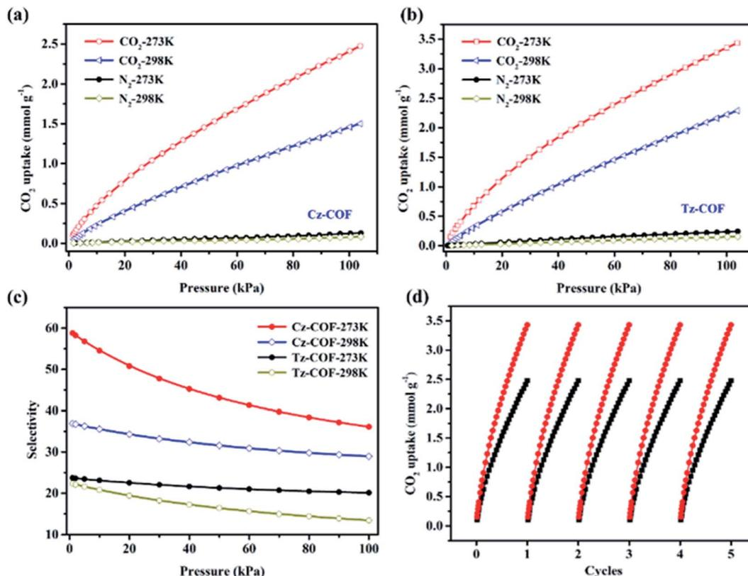
Fig. 3 CO<sub>2</sub> and N<sub>2</sub> adsorption isotherms for (a) Cz-COF and (b) Tz-COF measured at 273 K and 298 K, respectively. (c) The selectivity of functionalized COFs for CO<sub>2</sub> over N<sub>2</sub> obtained from the IAST method. (d) Cyclic CO<sub>2</sub> adsorption for functionalized COFs (black line, Cz-COF; red line, Tz-COF).
