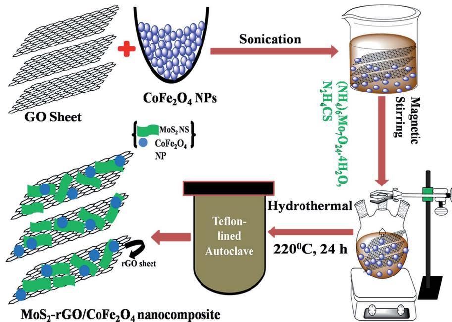
Fig. 1 Schematic illustration of the synthetic route to MoS<sub>2</sub>-rGO and the MoS<sub>2</sub>-rGO/CoFe<sub>2</sub>O<sub>4</sub> nanocomposite.
