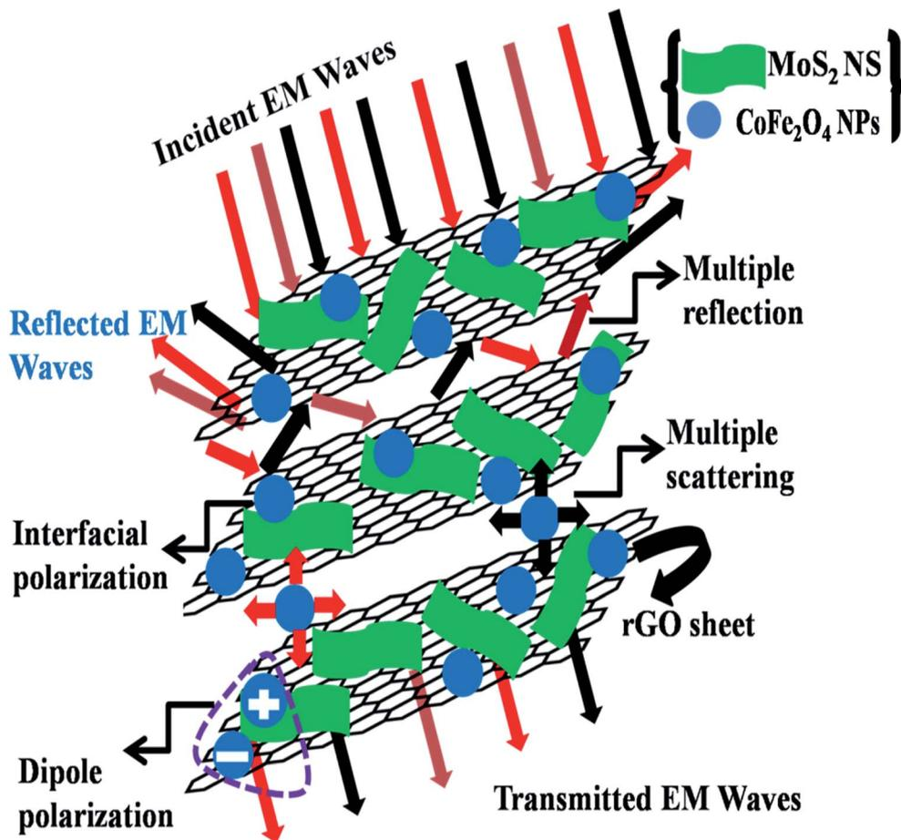
Fig. 8 A schematic illustration of the EMI shielding mechanism in the MoS<sub>2</sub>-rGO/CoFe<sub>2</sub>O<sub>4</sub> nanocomposite.
