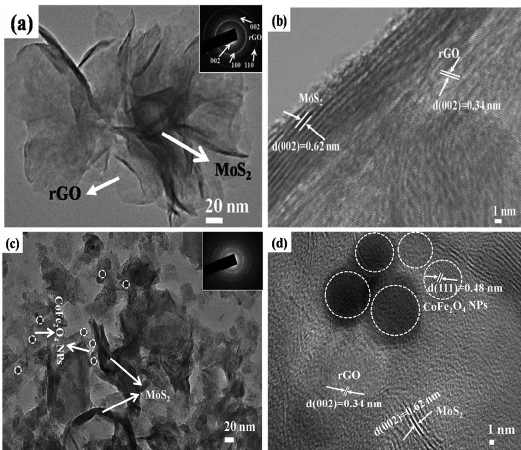
Fig. 5 TEM images of (a) MoS<sub>2</sub>-rGO and (c) MoS<sub>2</sub>-rGO/CoFe<sub>2</sub>O<sub>4</sub> at low-resolution and (b) MoS<sub>2</sub>-rGO and (d) MoS<sub>2</sub>-rGO/CoFe<sub>2</sub>O<sub>4</sub> at high-resolution.
