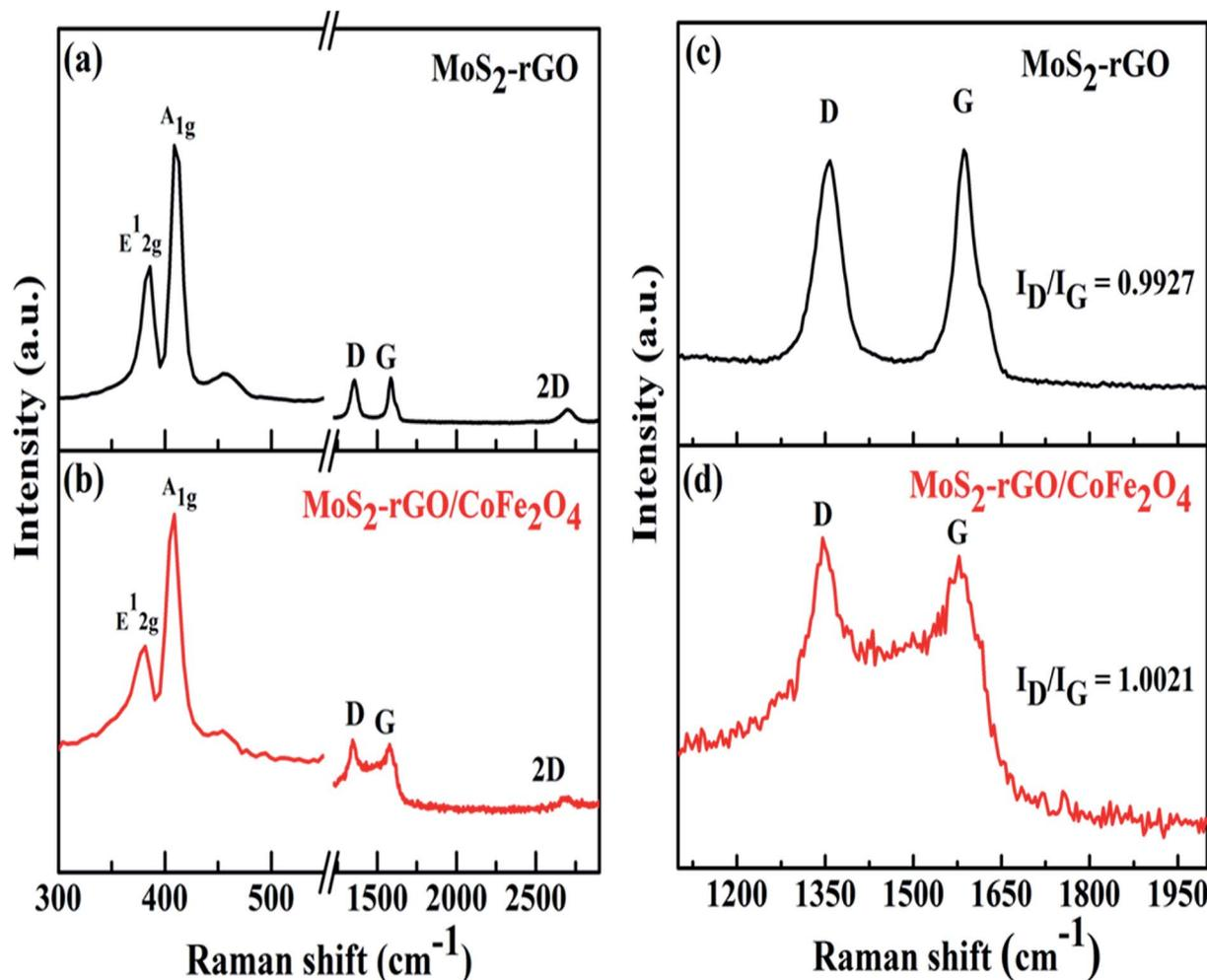
Fig. 3 Raman spectra of (a) MoS<sub>2</sub>-rGO, and (b) the MoS<sub>2</sub>-rGO/CoFe<sub>2</sub>O<sub>4</sub> nanocomposite, and (c) and (d) enlarged views of the D and G bands.
