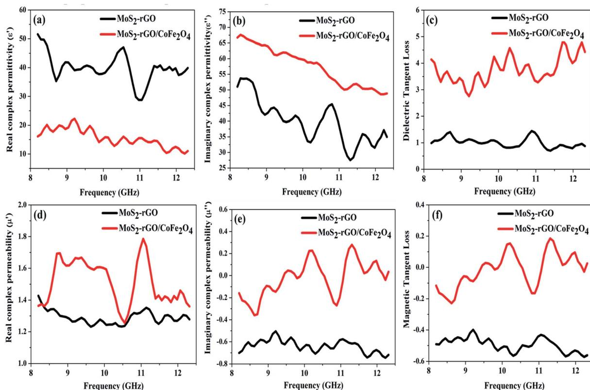
Fig. 7 Frequency dependence of the (a) and (b) complex permittivity, (d) and (e) complex permeability, and corresponding (c) dielectric loss tangent and (f) magnetic loss tangent of MoS<sub>2</sub>-rGO and the MoS<sub>2</sub>-rGO/CoFe<sub>2</sub>O<sub>4</sub> nanocomposite.
