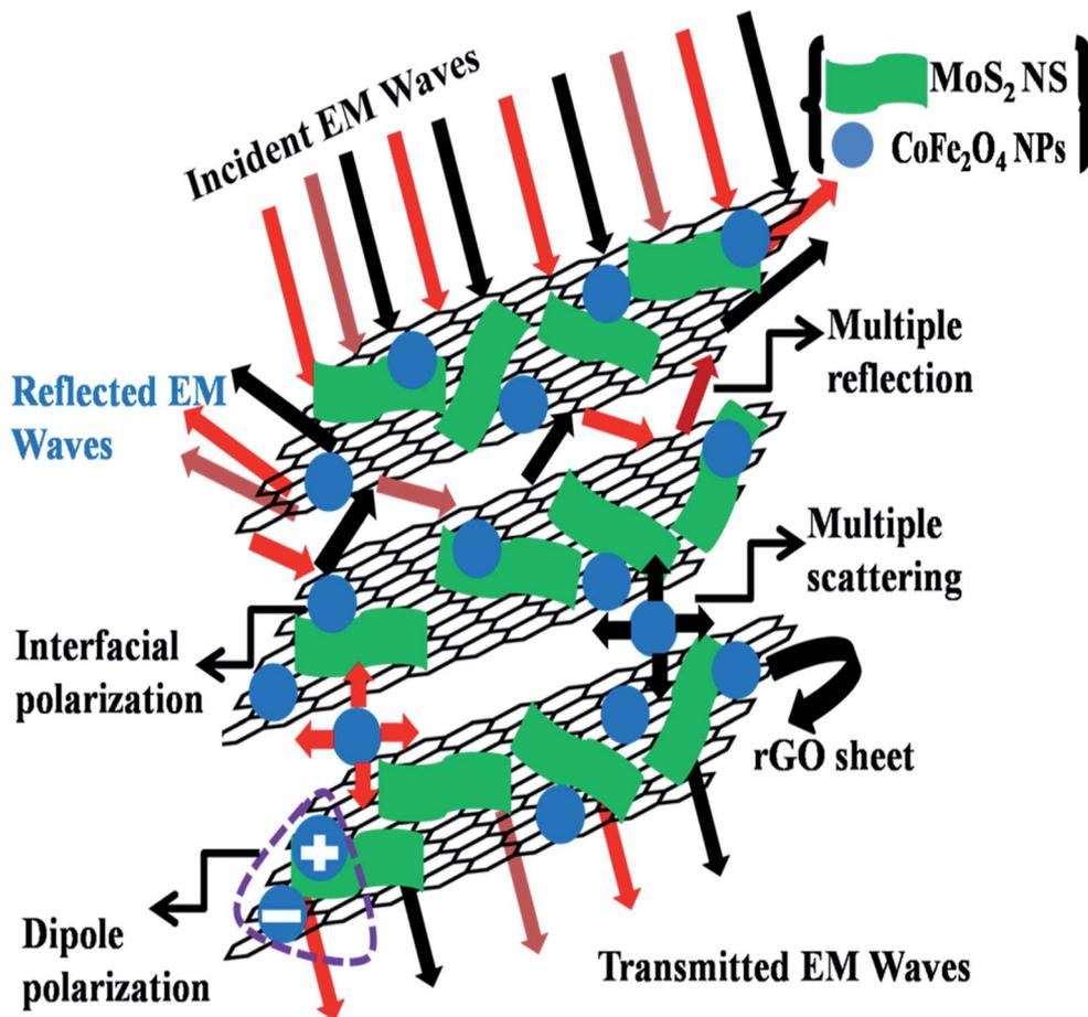
Fig. 8 A schematic illustration of the EMI shielding mechanism in the  $\text{MoS}_2\text{-rGO/CoFe}_2\text{O}_4$  nanocomposite.
