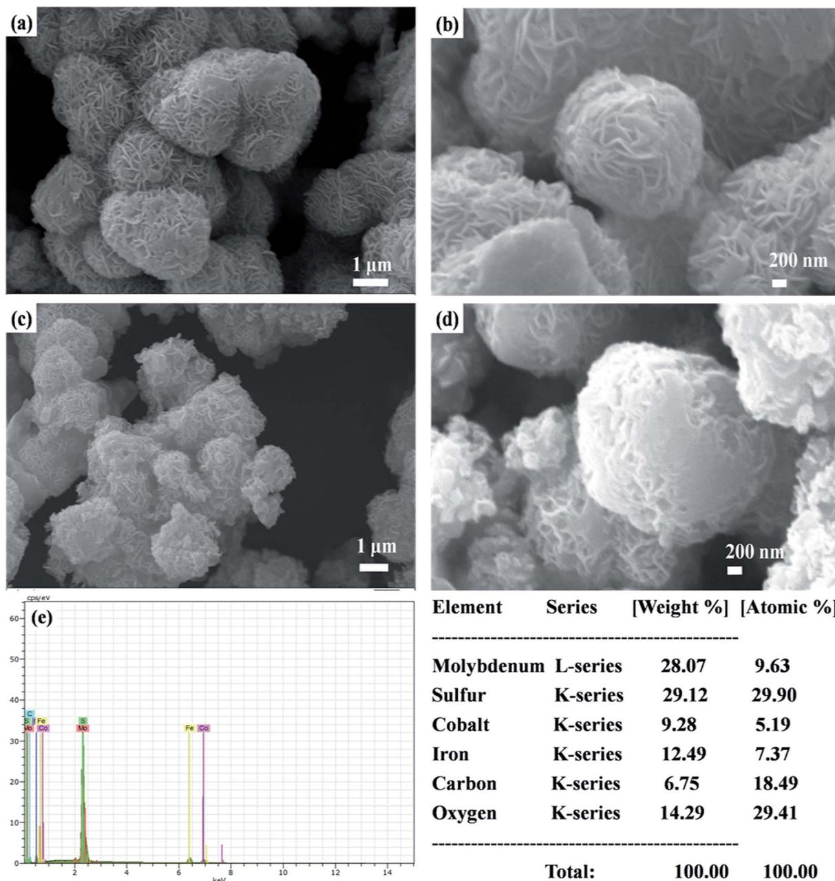
Fig. 4 Typical SEM pictures of as-prepared (a) MoS<sub>2</sub>-rGO and (c) the MoS<sub>2</sub>-rGO/CoFe<sub>2</sub>O<sub>4</sub> nanocomposite at low-magnification, and (b) MoS<sub>2</sub>-rGO and (d) MoS<sub>2</sub>-rGO/CoFe<sub>2</sub>O<sub>4</sub> at high magnification. (e) EDX data from the MoS<sub>2</sub>-rGO/CoFe<sub>2</sub>O<sub>4</sub> nanocomposite.
