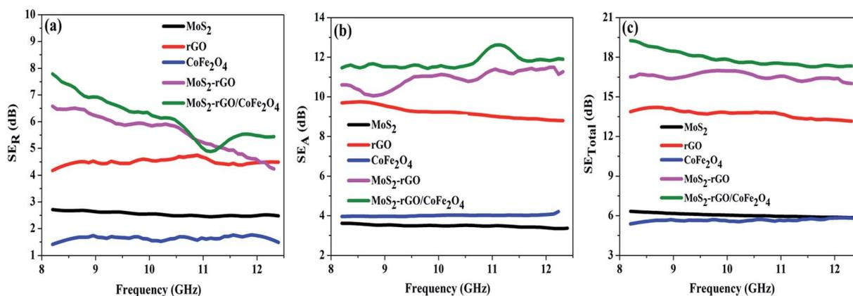
Fig. 6 Frequency dependence of the EMI shielding performance: (a)  $SE_R$ , (b)  $SE_A$ , and (c)  $SE_T$  values of MoS<sub>2</sub>, rGO, CoFe<sub>2</sub>O<sub>4</sub>, MoS<sub>2</sub>-rGO, and the MoS<sub>2</sub>-rGO/CoFe<sub>2</sub>O<sub>4</sub> nanocomposite in the X-band range.
