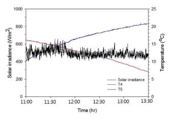
Fig. 8 Solar irradiation and the temperature rise of the pure water passing through Type 1 FPC. The experiment was carried out for 2.5 hours from 11:00 and the water temperature and the ambient air temperature were measured through T4 (the working fluid temperature) and T5 (the ambient temperature) shown in Fig. 7.
