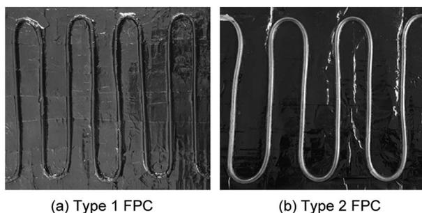
Fig. 6 Photos of the FPCs of Type 1 and Type 2. The copper tube of Type 1 is placed under the absorbing plate while the transparent urethane tube of Type 2 is placed on the absorbing plate. The absorbing plates made of copper tape were painted black although their colours in the photos do not appear completely black due to the light reflection on taking the pictures.
