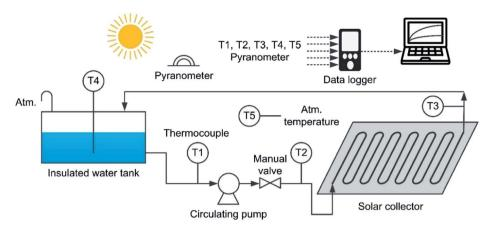
Fig. 7 Schematic diagram of the experimental apparatus. Although a flow control valve was installed to control the working fluid flowrate, it was fully opened during the experiment due to the insufficient pump capacity
