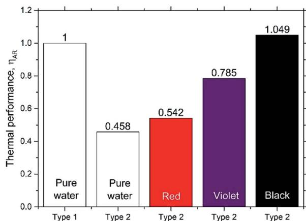
Fig. 11 Thermal performance based on the area ratio ( $\eta_{AR}$ ) of Type 1 and Type 2 FPCs. The thermal efficiency of Type 1 was set to 1.0 for comparison of the thermal efficiencies of Type 1 and Type 2 FPCs.
