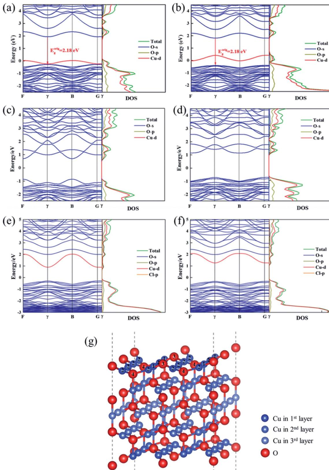
Fig. 2 Band structures and DOS of  $\text{Cu}_2\text{O}$  (111) with (a)  $V'_{\text{Cu-1}}$ ; (b)  $V'_{\text{Cu-2}}$ ; (c)  $V''_{\text{O-3}}$ ; (d)  $V''_{\text{O-4}}$ ; (e)  $\text{Cl}'_{\text{O-3}}$ ; (f)  $\text{Cl}'_{\text{O-4}}$ ; (g) side view of  $\text{Cu}_2\text{O}$  (111) slab model.
