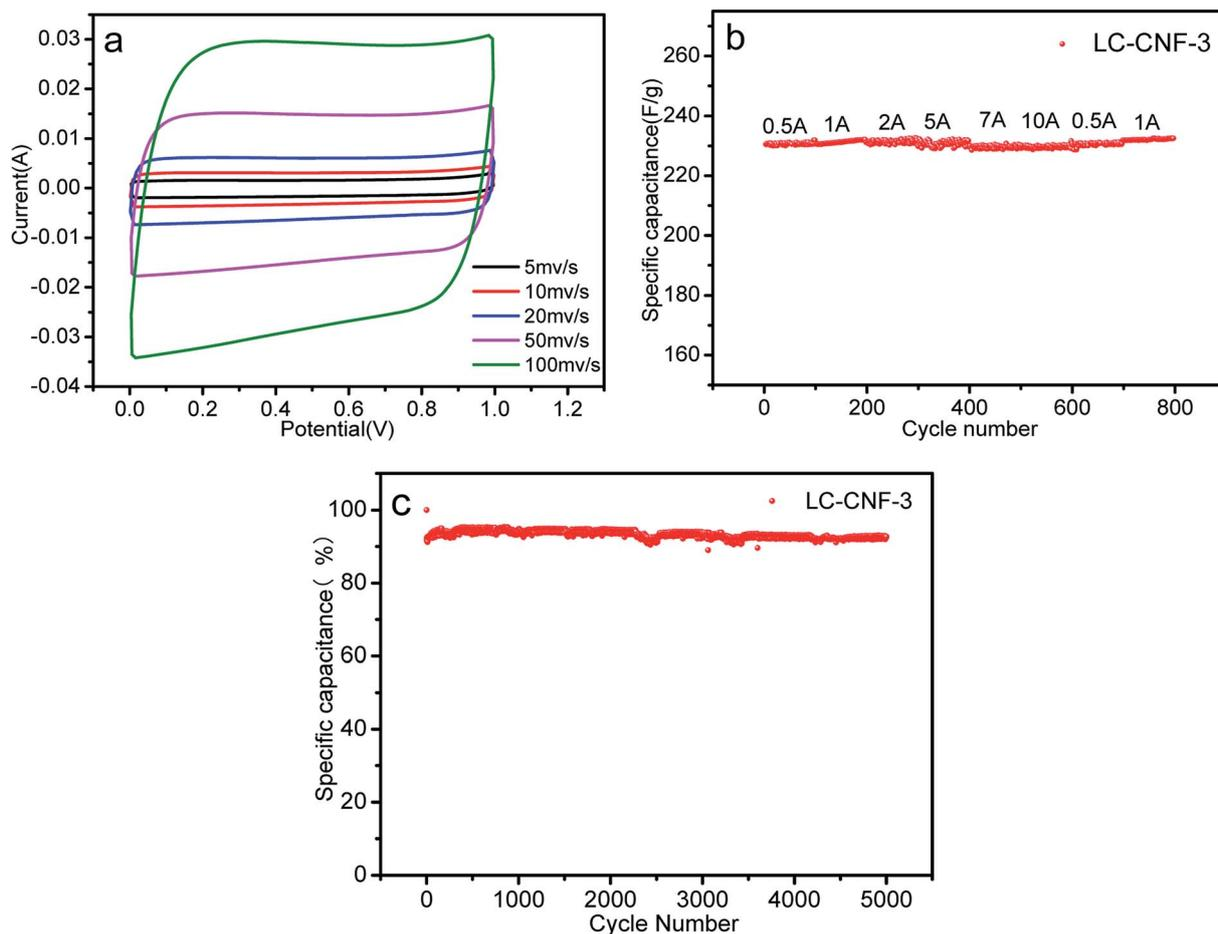
Fig. 8 (a) CV curves for the all-solid-state device at scan rates ranging from 5 to 100  $\text{mV s}^{-1}$ , (b) rate capability of the all-solid-state device, and (c) cycling stability performance of the all-solid-state device at a current density of 2  $\text{A g}^{-1}$  after 5000 cycles.
