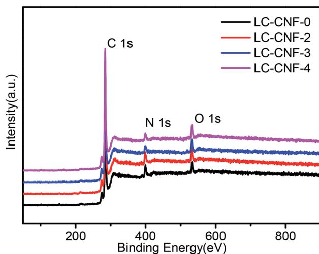
Fig. 5 XPS survey spectra of LC-CNF-0, LC-CNF-2, LC-CNF-3 and LC-CNF-4.
