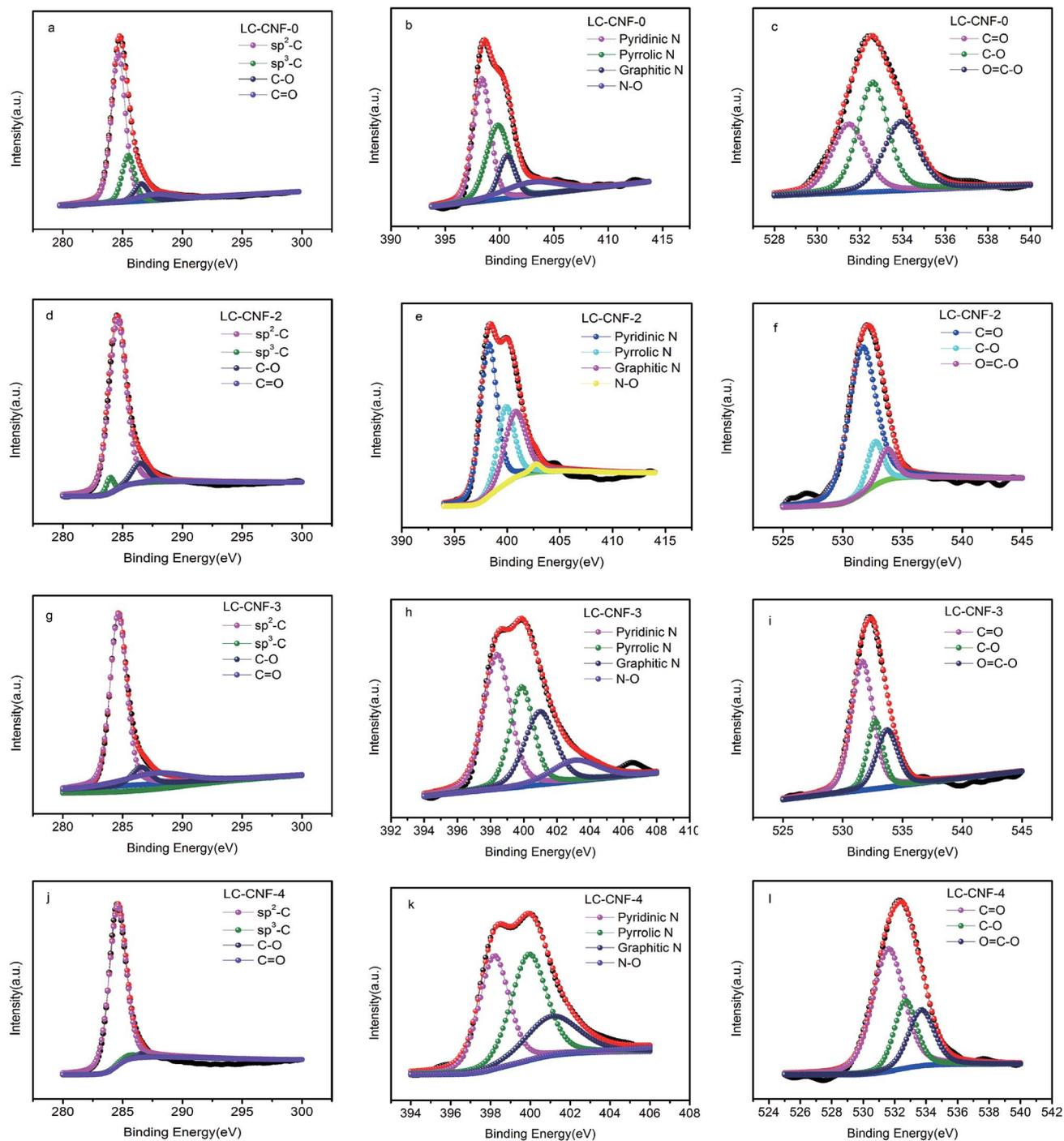
Fig. 6 XPS survey spectra of C 1s, O 1s, and N 1s orbitals for LC-CNF-0, LC-CNF-2, LC-CNF-3 and LC-CNF-4.
