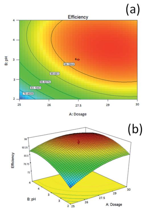
Fig. 10 Response surface of demulsification efficiency versus pH value and dosage of M-RGO6 (a) contour plot and (b) 3D surface.
