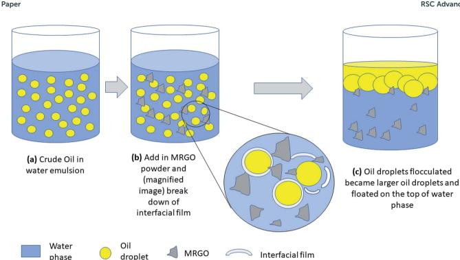
Fig. 11 Schematic diagram illustrated the demulsification process when M-RGO was added in the oil in water emulsion.
