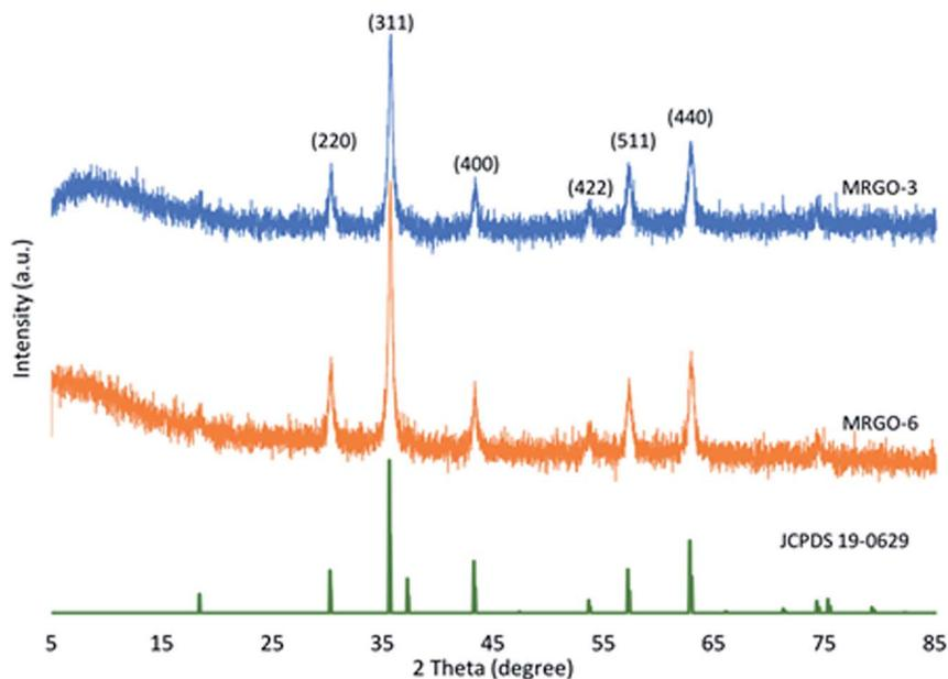
Fig. 1 XRD patterns of M-RGO3 and M-RGO6.
