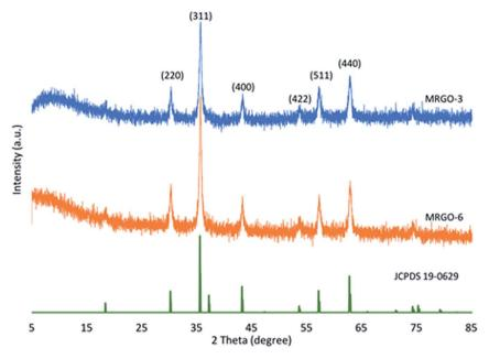
Fig. 1 XRD patterns of M-RGO3 and M-RGO6.
