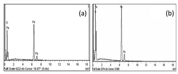
Fig. 6 EDX spectra of (a) M-RGO3 and (b) M-RGO6
