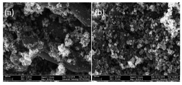
Fig. 4 FESEM image of (a) M-RGO3 and (b) M-RGO6.
