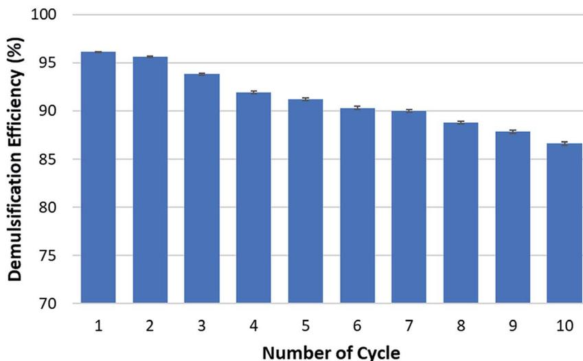
Fig. 12 Demulsification efficiencies of M-RGO nanocomposites in crude O/W emulsion for multiple cycle tests.
