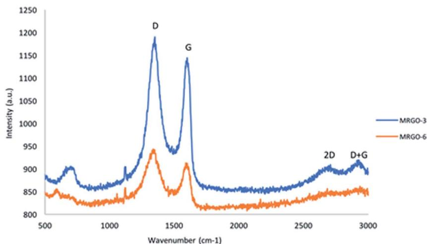
Fig. 7 Raman spectra of M-RGO3 and M-RGO6.
