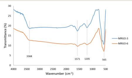
Fig. 2 FTIR spectra of M-RGO3 and M-RGO6.
