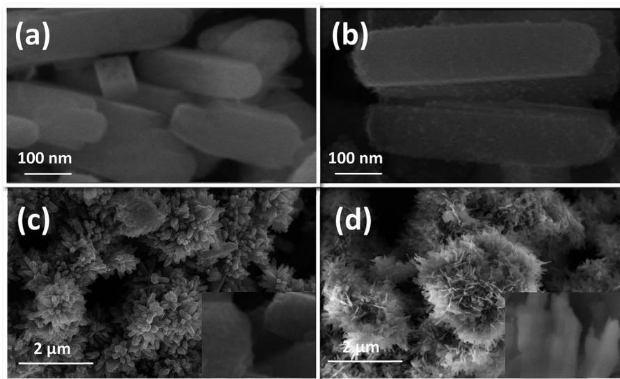
Fig. 2 NFO NRs prepared using  $\text{CO}(\text{NH}_2)_2$  and  $\text{NH}_4\text{F}$ , having molar ratios of (a) 1 : 1 and (b) 1 : 2, respectively, flowerlike morphology of NCF 1D NRs synthesized at (c) 120 and (d) 180 °C reaction temperatures. Insets show edges of the respective NRs.
