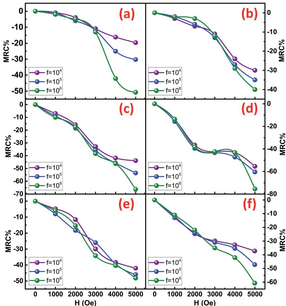
Fig. 10 MRC% at different magnetic field (H) for (a) CFO-1, (b) CFO-2, (c) NFO-1, (d) NFO-2, (e) NCF-1 and (f) NCF-2 NRs.
