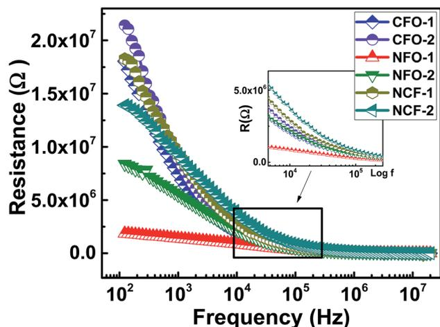
Fig. 8 Dispersion of resistance ( $R$ ) vs. frequency for ferrite NRs synthesized at different reaction temperatures. Inset shows the magnified image of dispersive curve elaborating different relaxation behavior.
