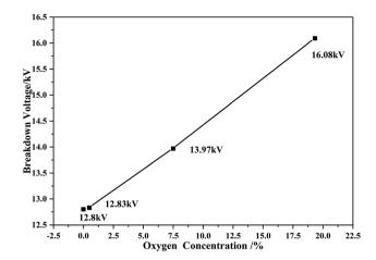
Fig. 3 Relationship between the oxygen concentration and breakdown voltage of  $C_5F_{10}O/N_2/O_2$ .
