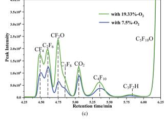
Fig. 6 Components after 60 times breakdown with different oxygen concentrations.
