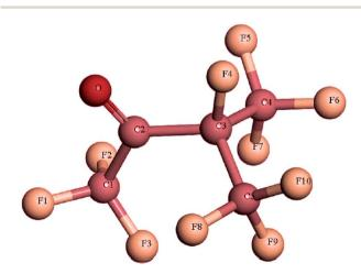
Fig. 1 Molecular structure of  $C_5F_{10}O$ .
