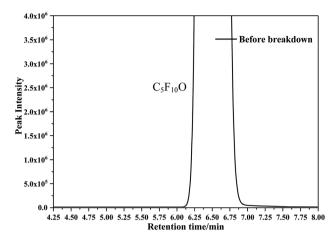
Fig. 5 Components before breakdown.
