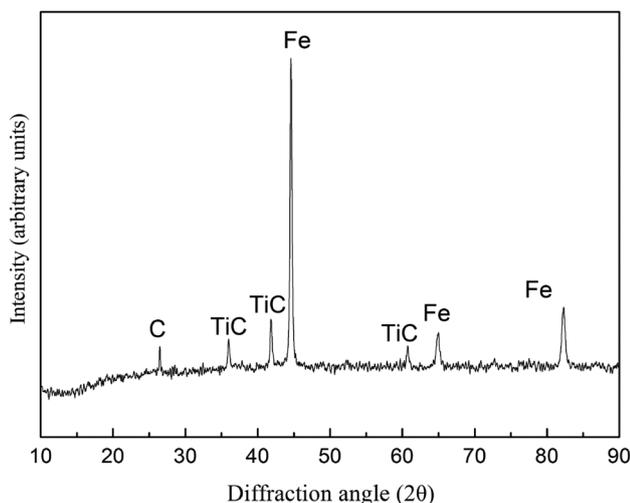
Fig. 5 XRD pattern of the sintered sample without rare-earth oxide.
