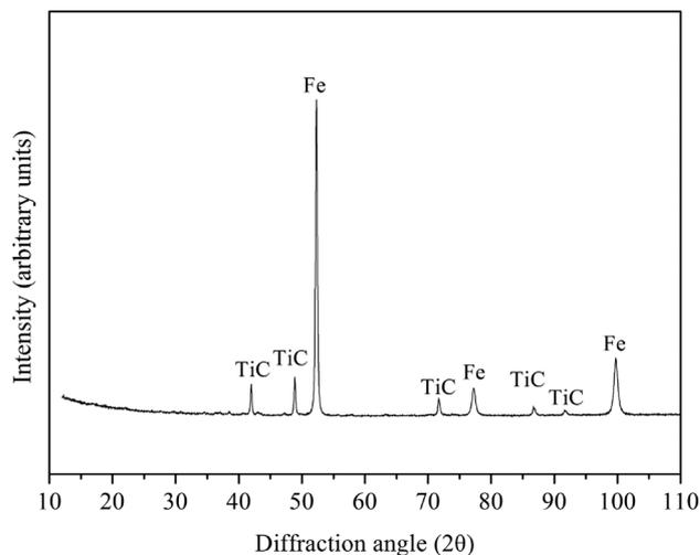
Fig. 2 XRD analysis of the pre-reduced powders.
