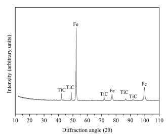
Fig. 2 XRD analysis of the pre-reduced powders.
