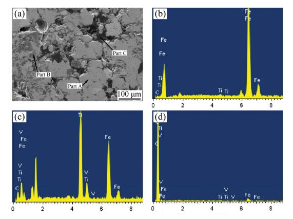
Microstructure of sintered sample (a) and EDS analysis of area A (b), B (c) and D (d)
