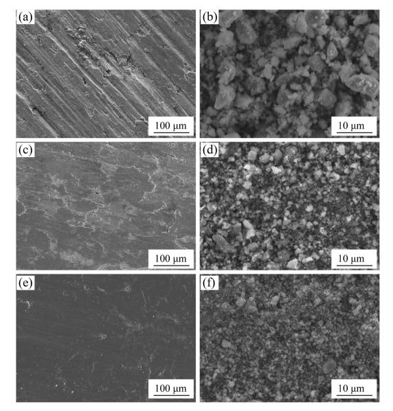
Fig. 10 Worn surface and wear debris of sintered samples. (a) and (b) without rare-earth oxide, (c) (d) La-0.2 wt%, and (e) and (f) Ce-0.4.
