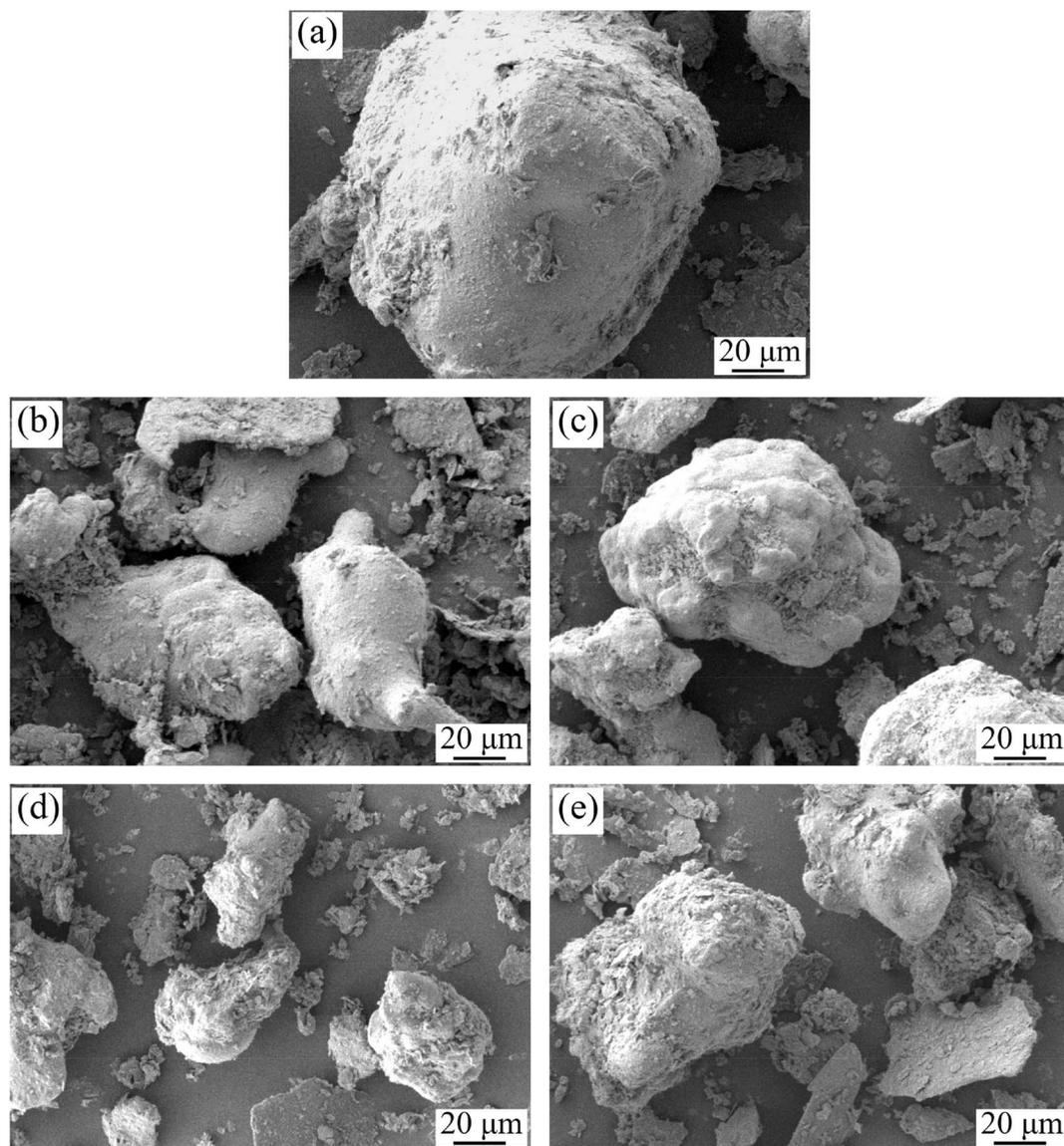
Fig. 6 SEM micrographs of powders (a) without and with (b) 0.2 wt%  $\text{La}_2\text{O}_3$ , (c) 0.4 wt%  $\text{La}_2\text{O}_3$ , (d) 0.4 wt%  $\text{CeO}_2$  and (e) 0.6 wt%  $\text{CeO}_2$ .
