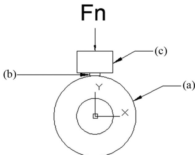
Fig. 3 Diagram of block-on ring tester (a) grinding wheel, (b) specimen, and (c) load.
