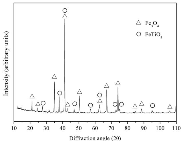
Fig. 1 XRD analysis of vanadium-bearing titanomagnetite concentrates.
