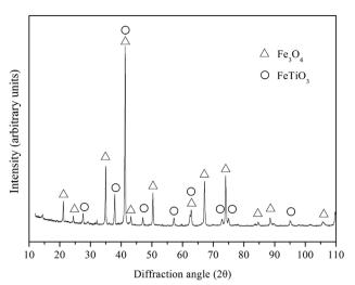
Fig. 1 XRD analysis of vanadium-bearing titanomagnetite concentrates.
