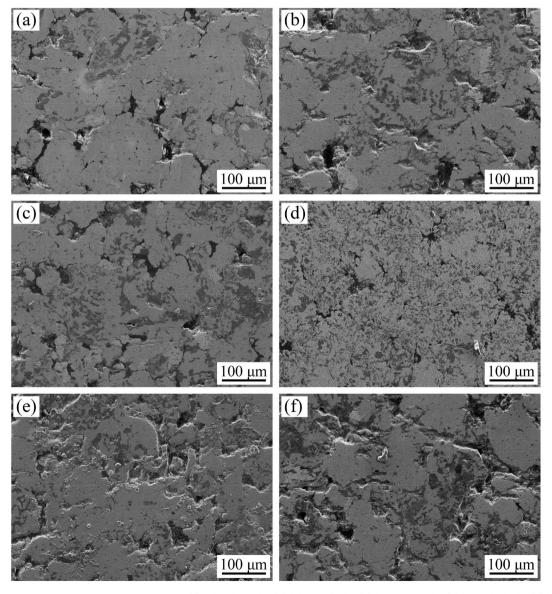
Fig. 7 Microstructure of the sintered specimens with (a) 0.2 wt% La<sub>2</sub>O<sub>3</sub>, (b) 0.2 wt% CeO<sub>2</sub>, (c) 0.4 wt% La<sub>2</sub>O<sub>3</sub>, (d) 0.4 wt% CeO<sub>2</sub>, (e) 0.6 wt% La<sub>2</sub>O<sub>3</sub>, (f) 0.6 wt% CeO<sub>2</sub>.
