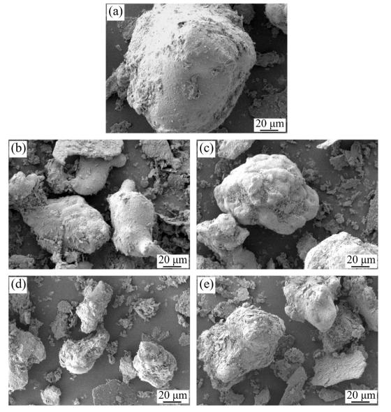
Fig. 6 SEM micrographs of powders (a) without and with (b) 0.2 wt% La<sub>2</sub>O<sub>3</sub>, (c) 0.4 wt% La<sub>2</sub>O<sub>3</sub>, (d) 0.4 wt% CeO<sub>2</sub> and (e) 0.6 wt% CeO<sub>2</sub>.
