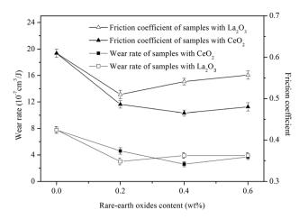
Fig. 9 Wear rate and friction coefficient of Fe-based friction material with different rare earth addition.
