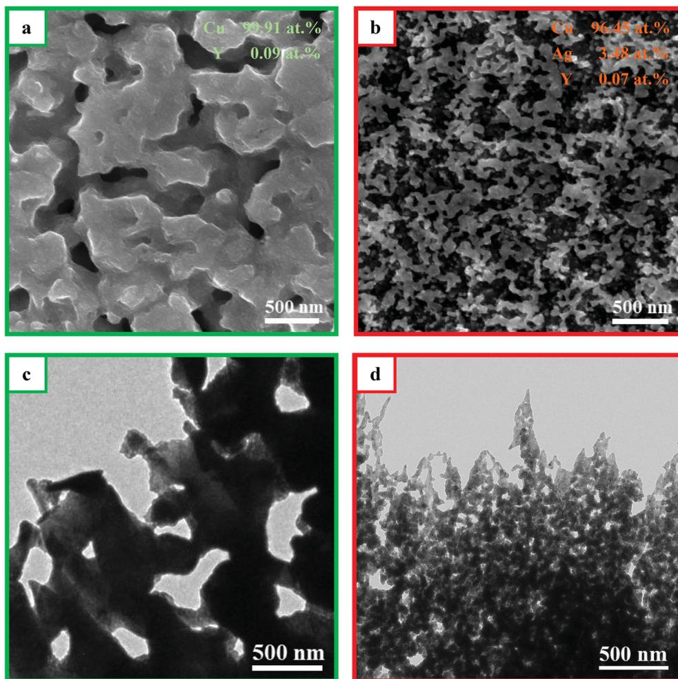
Fig. 2 SEM images of the samples prepared by dealloying (a)  $\text{Cu}_{72}\text{Y}_{28}$  and (b)  $\text{Cu}_{70}\text{Y}_{28}\text{Ag}_2$  metallic glasses in 1 M  $\text{H}_2\text{SO}_4$  aqueous solution at 333 K for 90 min. TEM images of the samples: (c) NPC; (d) NPCS.
