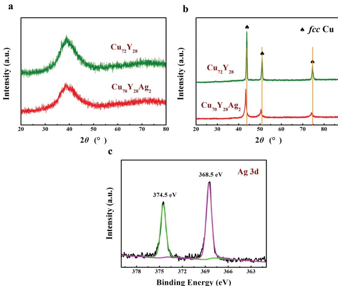
Fig. 1 XRD patterns of (a) Cu–Y(–Ag) metallic glasses and (b) the corresponding samples after dealloying in 1 M  $\text{H}_2\text{SO}_4$  aqueous solution at 333 K for 90 min; (c) XPS Ag 3d spectra of as-dealloyed  $\text{Cu}_{70}\text{Y}_{28}\text{Ag}_2$  ribbons.
