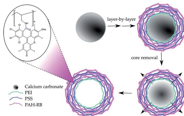
Scheme 1 Preparation of hollow microcapsules (HM) using layer by layer self-assembly technique onto CaCO<sub>3</sub> template. Inset: proposed molecular structure of the PAH-RB polycation.
