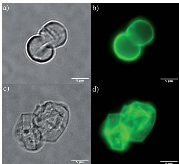
**Fig. 4** Optical (a and c) and fluorescence (b and d) microscopy images of microcapsules with  $\text{CaCO}_3$  (a and b) and after the dissolution of the mold with EDTA (c and d). Excitation was at 545 nm and emission was collected at 605 nm. The image color does not correspond to the light emitted by the sample. It was digitally colored post-acquisitions.
