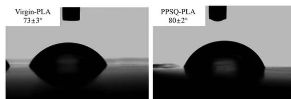
Fig. 9 Water contact angle of virgin-PLA and PPSQ-PLA.
