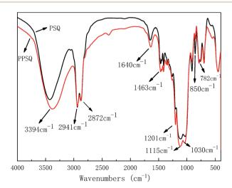
Fig. 2 The FT-IR curves of PSQ and PPSQ.
