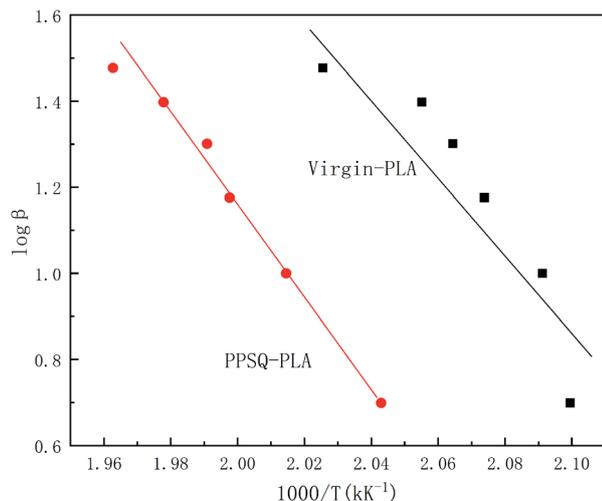
Fig. 5 The curves fitting of  $\log \beta$  vs.  $1/T$  with Ozawa method.
