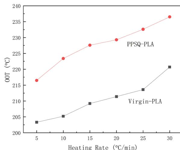
Fig. 4 The OOT values of virgin-PLA and PPSQ-PLA at different heating rates.
