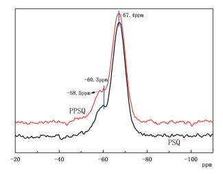
Fig. 1 Solid-state NMR spectra of PSQ and PPSQ.
