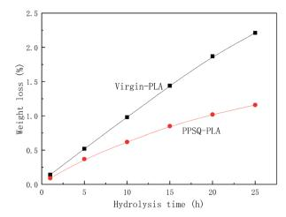
Fig. 7 Weigh loss of virgin-PLA and PPSQ-PLA at different hydrolysis time.
