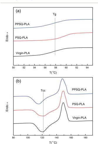
Fig. 3 The melting curve of virgin-PLA, PSQ-PLA and PPSQ-PLA.
